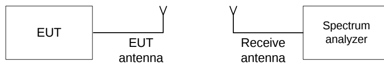
Figure 7.7.1 Band edge emission test setup
