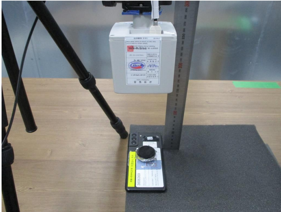
Top charger below client (20cm distance)
