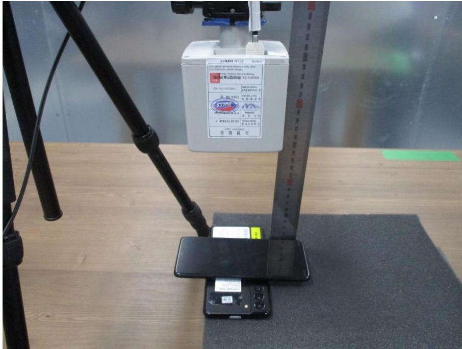
Top charger below client (20cm distance)
