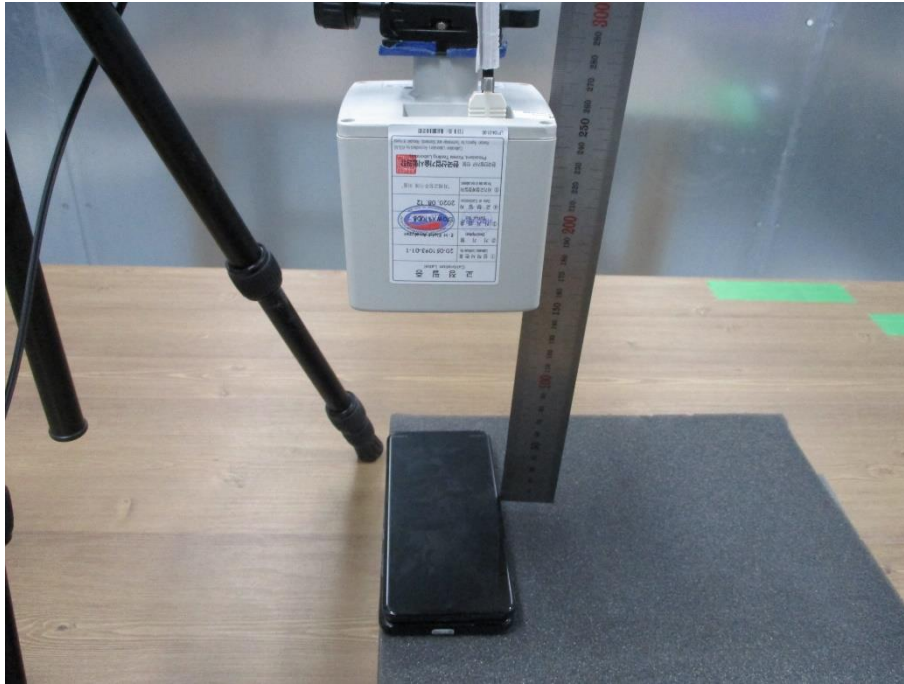
Top charger below client (20cm distance)
