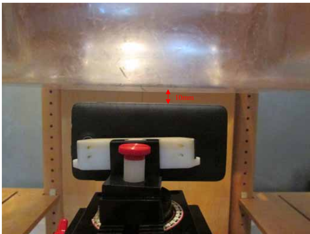
Body-worn Left Setup Photo (10mm)
