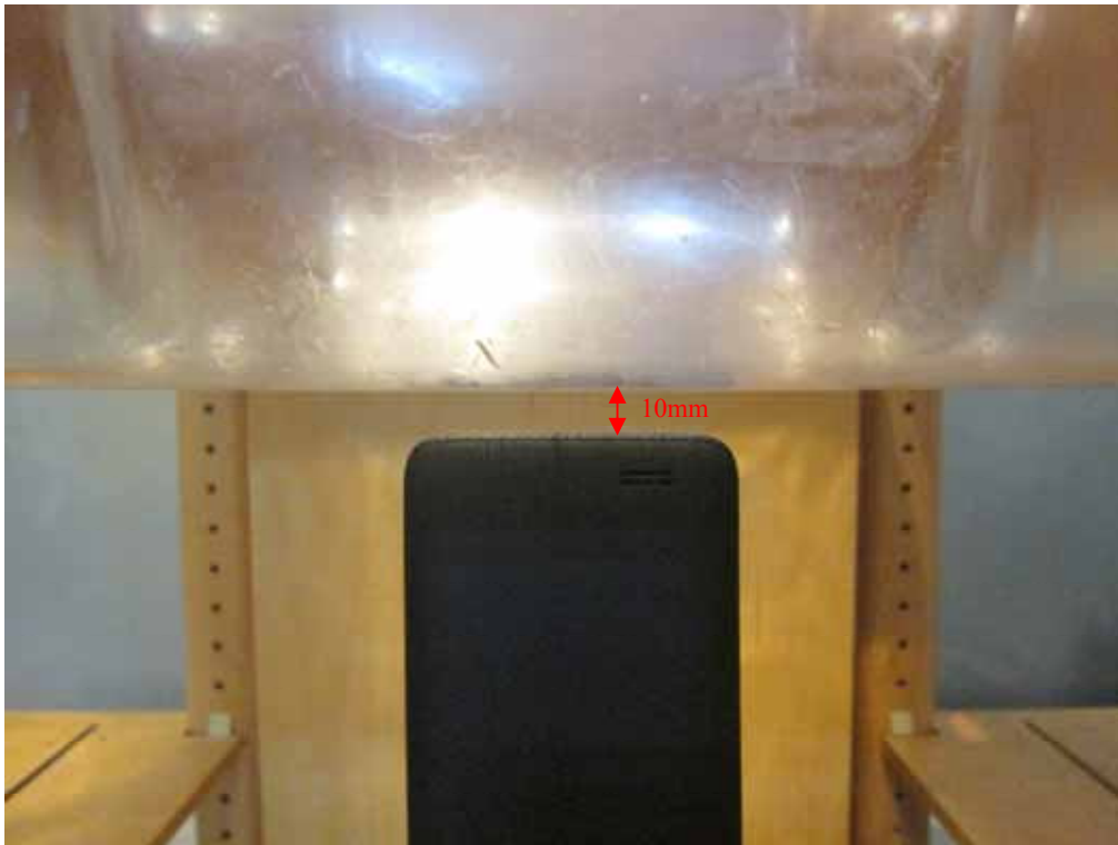
Body-worn Bottom Setup Photo (10mm)
