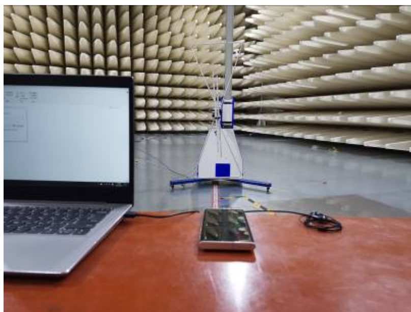
Radiated Emissions Test Setup (30-1000MHz)
