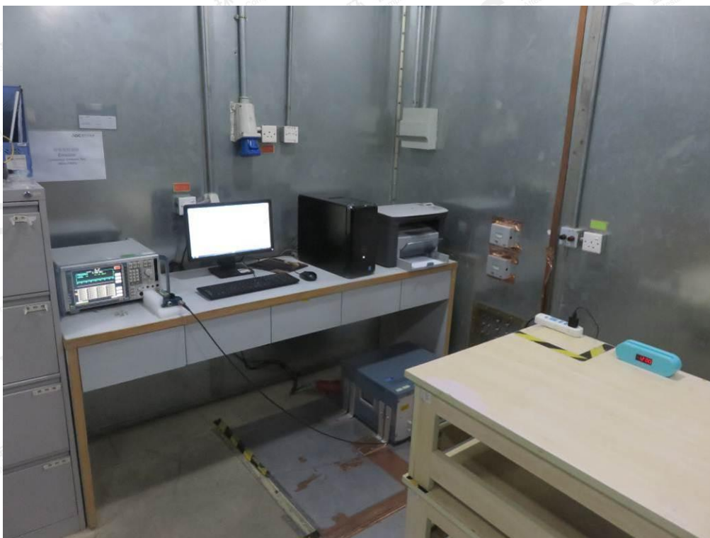
FCC RADIATED EMISSION TEST SETUP
