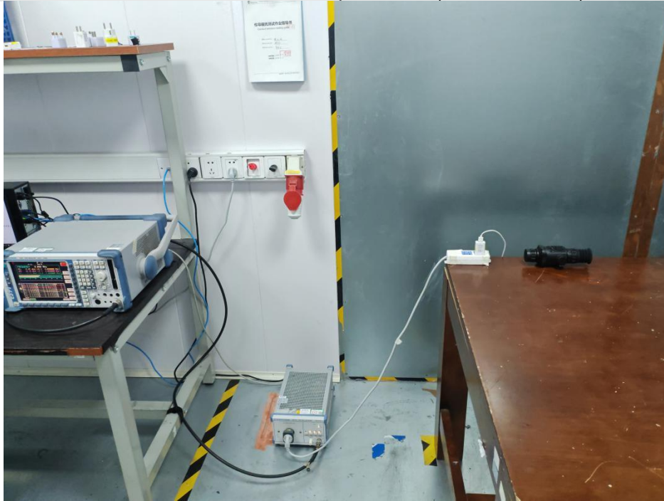
Conducted emissions at AC power line (150kHz-30MHz)
