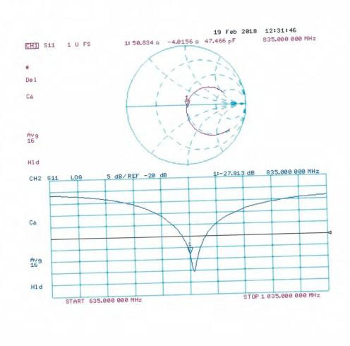
Impedance Measurement Plot for Head TSL
