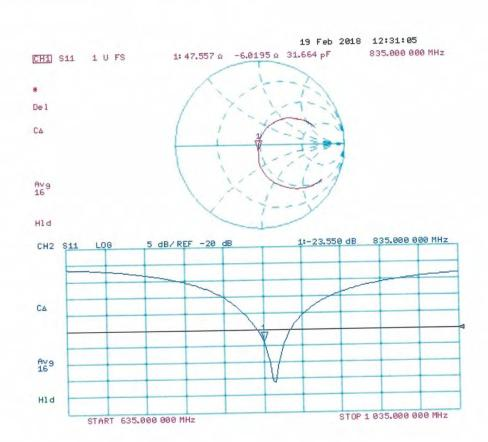
Impedance Measurement Plot for Body TSL
