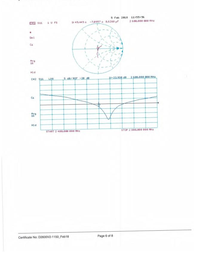
Impedance Measurement Plot for Head TSL
