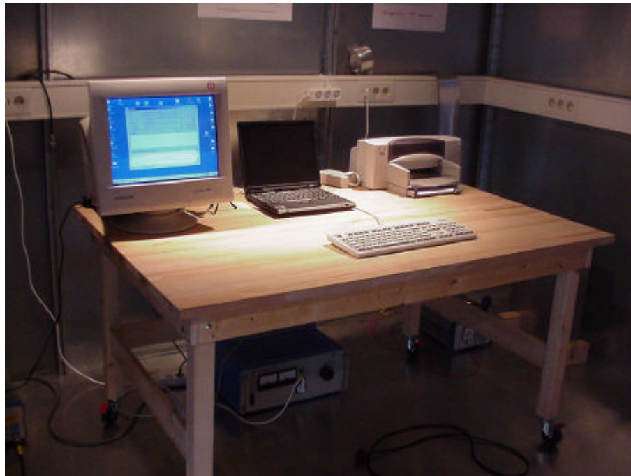
Picture 3 : Setup for emission measurement on the AC mains
