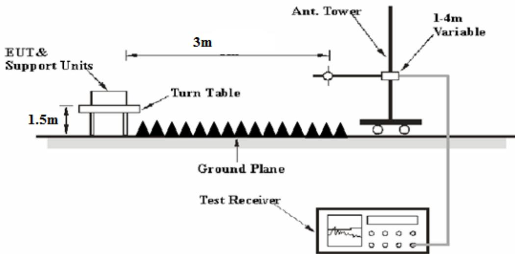
The radiated emission below 1GHz tests were performed in the 10 meters chamber test site, above 1GHz tests were performed in the 3 meters chamber test site A, using the setup accordance with the ANSI C63.10-2013. The specification used was the FCC 15.209, and FCC 15.249 limits.
