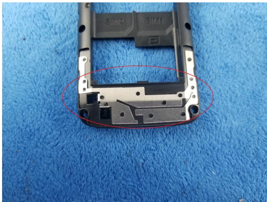
GSM/PCS - Antenna View
