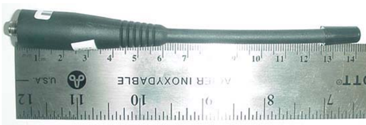
Quarter-Wave Whip Antenna (P/N: 501-0017-107)
