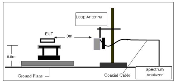
2. Radiated Emission Test-Up Frequency 30MHz~1GHz
