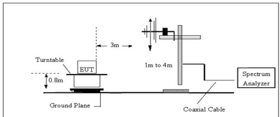
3. Radiated Emission Test-Up Frequency Above 1GHz
