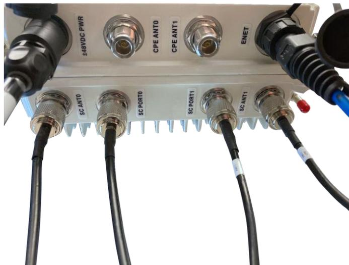
3. Remove the protective caps from GM02 Mesh Node Type-N RF Connector Ports labeled “CPE ANT0” and “CPE ANT1” and connect Type-N Patch Cables from these connectors to the input ports of the Backhaul Antenna. Tighten Type-N Connectors to 12 in-lbs. +/- 10% (1.36 N-m +/- 10%).
