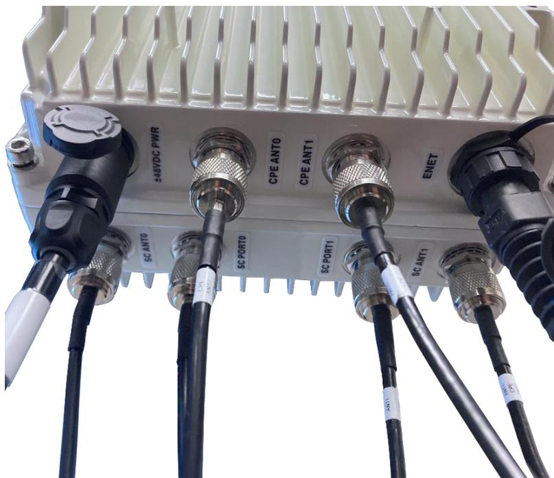
4. Seal each of the RF Connectors using Cold Shrink, Heat Shrink, Self-Fusing (Butyl) Tape, or similar, wrapping each from the Mesh Node to approximately 1 inch below the ferrule heat shrink of the cable or similar.
