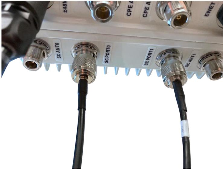
2. Remove the protective caps from the GM02 Mesh Node Type-N RF Connector Ports labeled “SC ANT0” and “SC ANT1” and connect Type-N Patch Cables from these connectors to the input ports of the Sector Antenna (antenna providing CBRS cellular coverage for the sector). Tighten Type-N Connectors to 12 in-lbs. +/- 10% (1.36 N-m +/- 10%).
