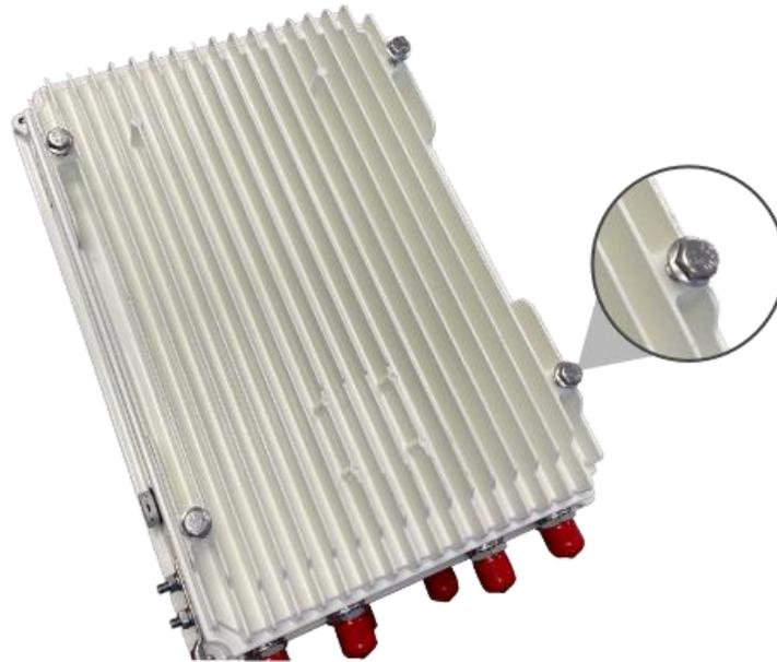
2. Loosen each of the M6 flange bolts to make sure that at least 3/16" (4mm) of gap exists between the casting of the Mesh Node unit and the underside of the washer of the M6 Flange Bolts.
