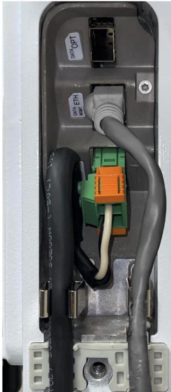
13. Close the wiring cavity and tighten the hex screw with a 5mm Allen wrench when the Ethernet and power connections from the GM02 to the AP are completed.
