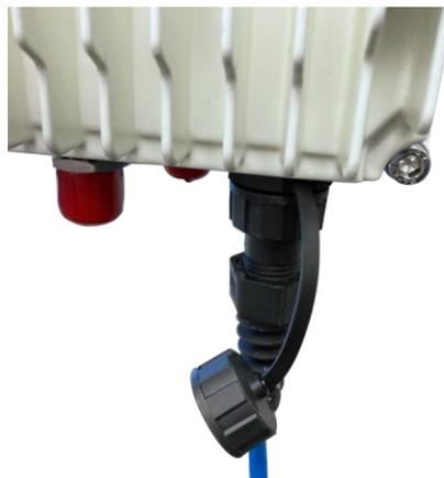
9. Route the other end of the cable into the Mesh AP wiring cavity and terminate it with an appropriate shielded RJ45 plug.
