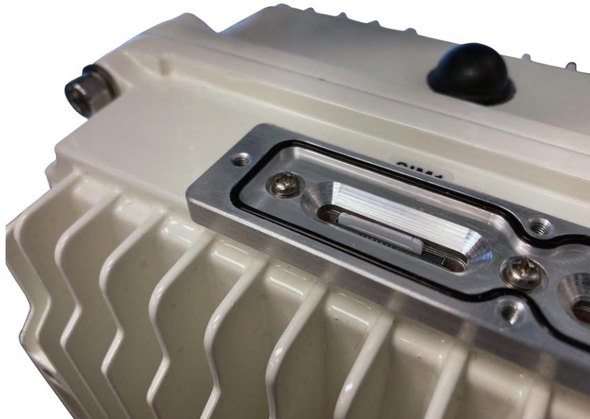
7. Replace cover and tighten the four M3 Captive Screws. Torque the M3 Captive Screws to 4 in-lbs. +/- 10% (0.45 N-m +/- 10%). Do not over torque screws.
