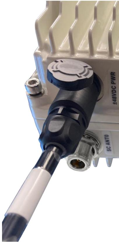
12. Open the G501 AP wiring cavity with a 5mm Allen wrench, route the AP power cable (green connector) through the left-side wire groove, and plug it into the PWR interface.
