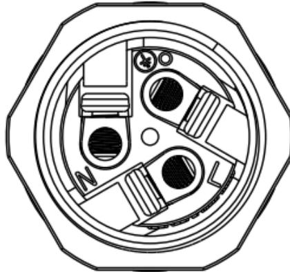
4. Insert the White Wire of the Lightning Suppressor Cable into the Line Contact (L) of the Connector of the Weathertight Cable Joiner and tighten the cable clamp screw to 1.8 to 3.5 in-lbs. (0.2 to 0.4 N-m).
