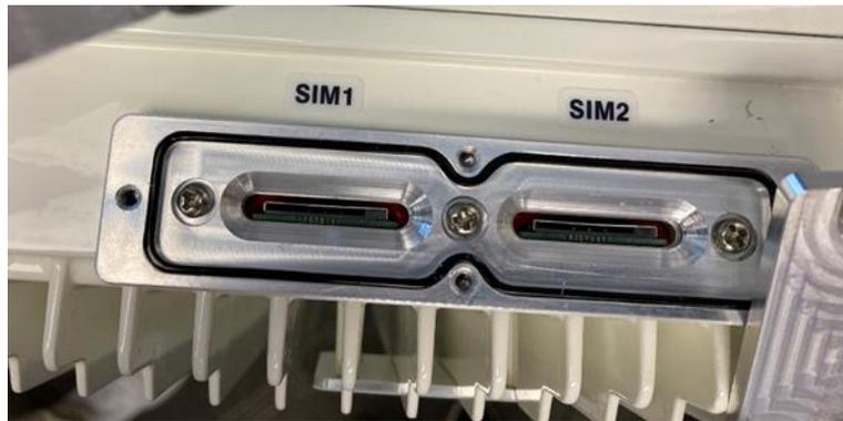
4. Insert standard size SIM Card into SIM Socket 1 in the orientation shown with its contacts facing the front of the unit and the trimmed corner (notch) oriented in the lower-left corner, as shown below. Ensure that card is inserted straight into socket. If significant resistance is felt, remove the SIM card, realign, and insert it into the socket again.
