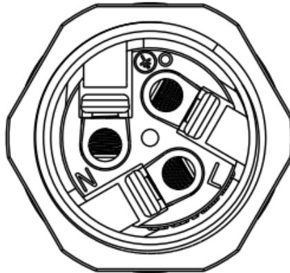
5. Insert the White Wire of the Power Cable into the Line Contact (L) of the Connector of the Weathertight Cable Joiner and tighten the cable clamp screw to 1.8 to 3.5 in-lbs. (0.2 to 0.4 N-m).
