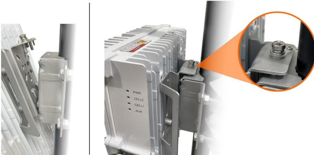
2. Tighten the screw on the top of the bracket using a Phillips (crosshead) screwdriver to complete the mounting procedure.
