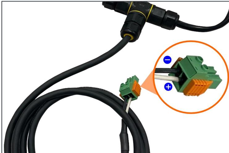
**NOTE:** The color of the conductors may vary. If the conductors are red/black, insert the red conductor into the + terminal and insert the black conductor into the - terminal. If the conductors are brown/blue, insert the brown conductor into the + terminal and insert the blue conductor into the - terminal.
