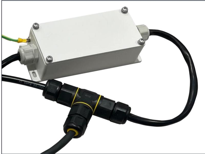
9. Assemble the Mesh AP Power Terminal. Insert the white conductor into the + terminal and insert the black conductor into the - terminal and tighten both terminal screws as shown in Figure 43.
