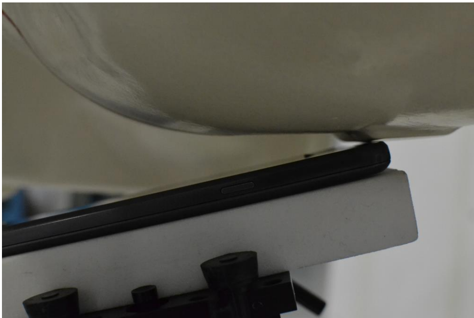
SAR Test Setup Photo 4 – Left Tilt
