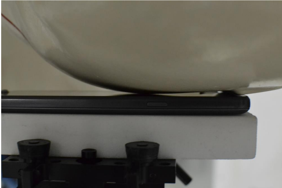
SAR Test Setup Photo 3 – Left Cheek
