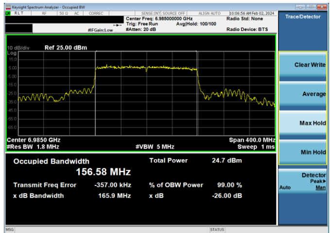
Plot 7-128. 26dB & 99% Bandwidth Plot Antenna WF8 (160MHz 802.11ax RU996x2 (UNII Band 8) – Ch. 207)
