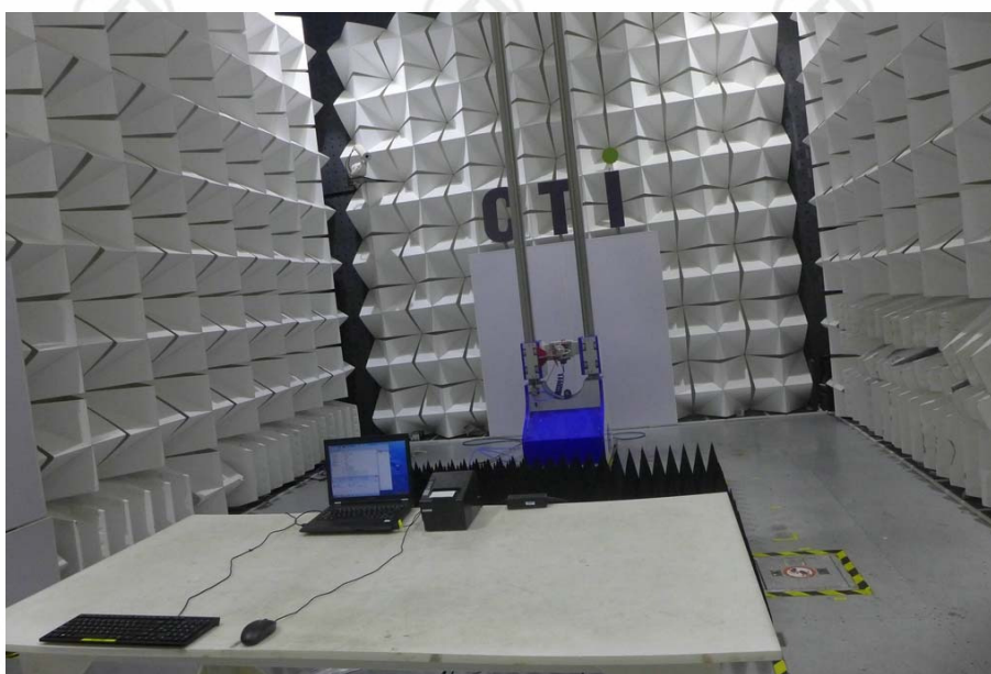
Radiated spurious emission Test Setup-3(Above 1GHz)
