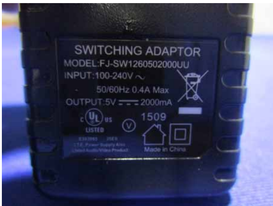
EUT – Adapter Label View
