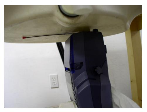
**Top Side 1.5cm Separation 1900MHz (Antenna 1)**
