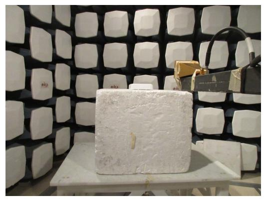
1.8 Radiated Spurious Emission 18-26.5 GHz at 1 meters Rear View
