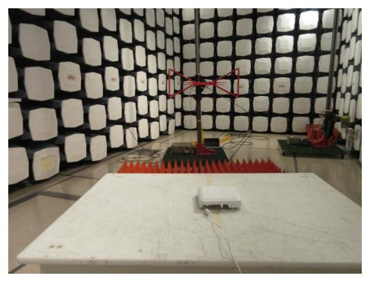
1.3 Radiated Spurious Emission 1-18 GHz at 3 meters Front View
