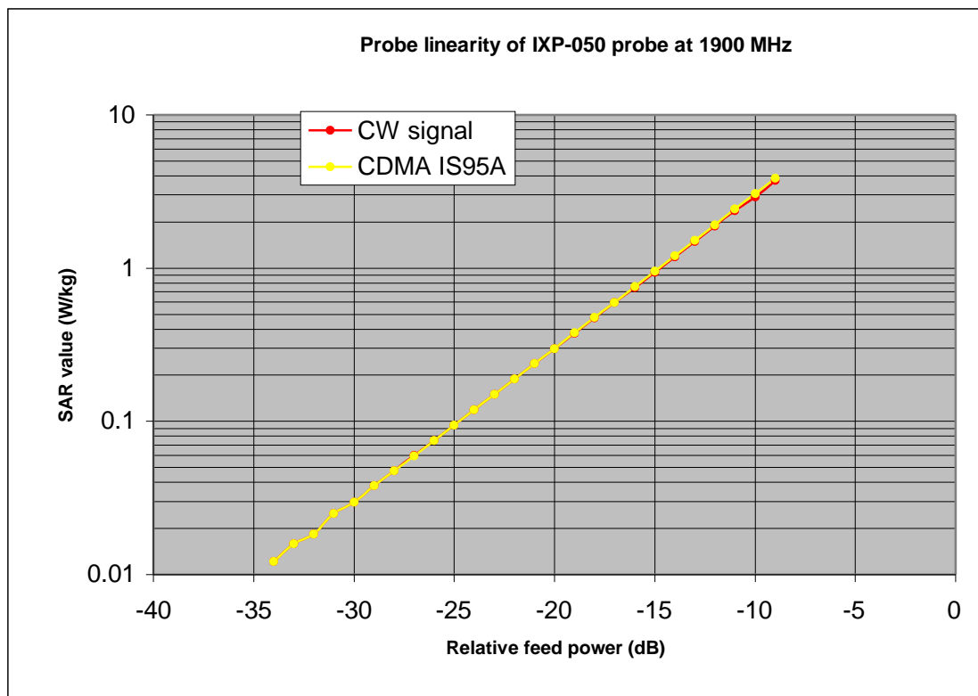
Figure 10. The CDMA response of an IXP-050 probe at 1900MHz.
