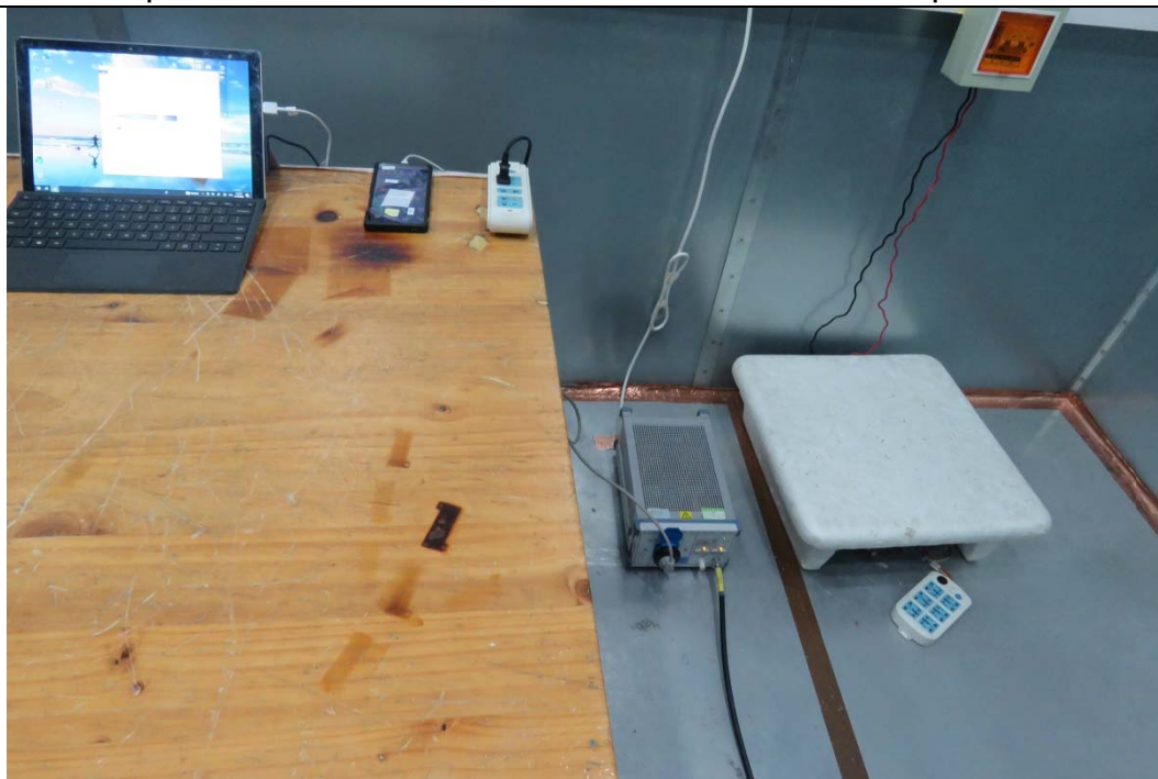
Picture 2: Conducted Emissions Test Setup
