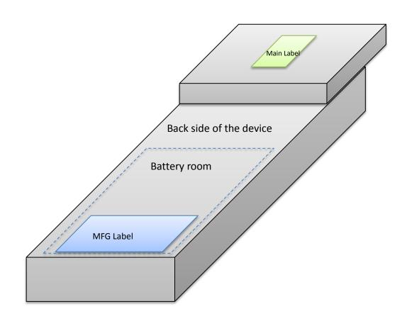
MFG label is in battery room. It is visible to the users as they install the battery.
