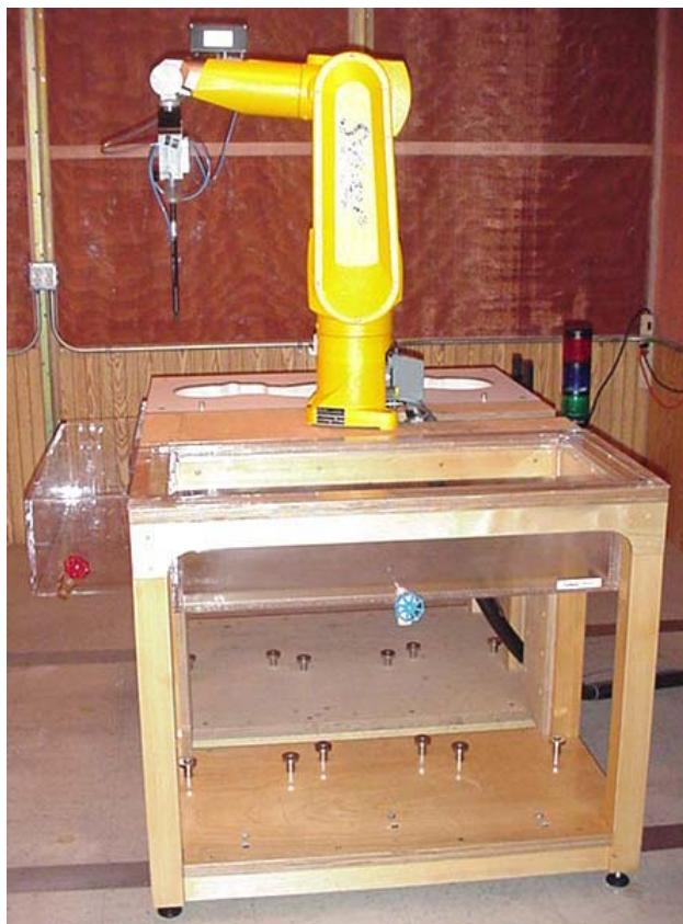
DASY4 SAR Measurement System with validation phantom
