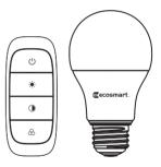
□ To unpair the LED Bulb with the remote, hold down the ON/OFF button () (BB) and the Customize White Light button () (DD) at the same time for 3 seconds. The indicator light (AA) will flash as it attempts to detect the LED Bulb. Once detected, the indicator light (AA) will flash rapidly indicating the unpairing process is underway.
