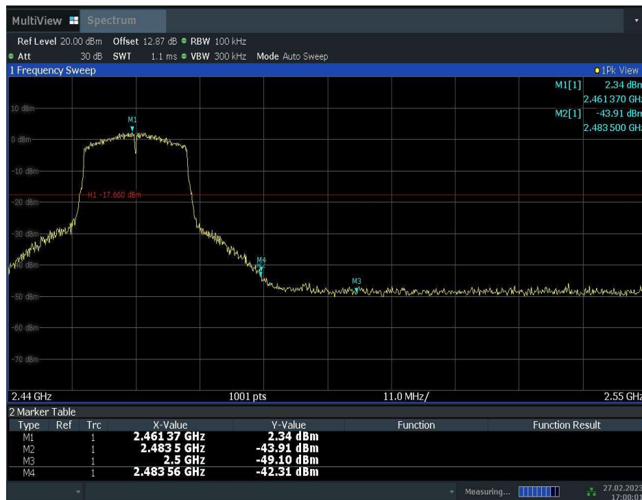
Fig.A.5.6 Band Edges (802.11n-HT20, Ch 11)
