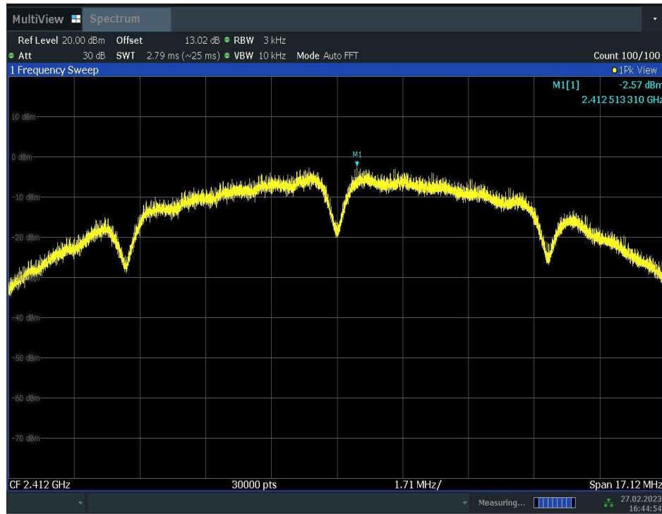
Fig.A.3.1 Power Spectral Density(802.11b,Ch1)
