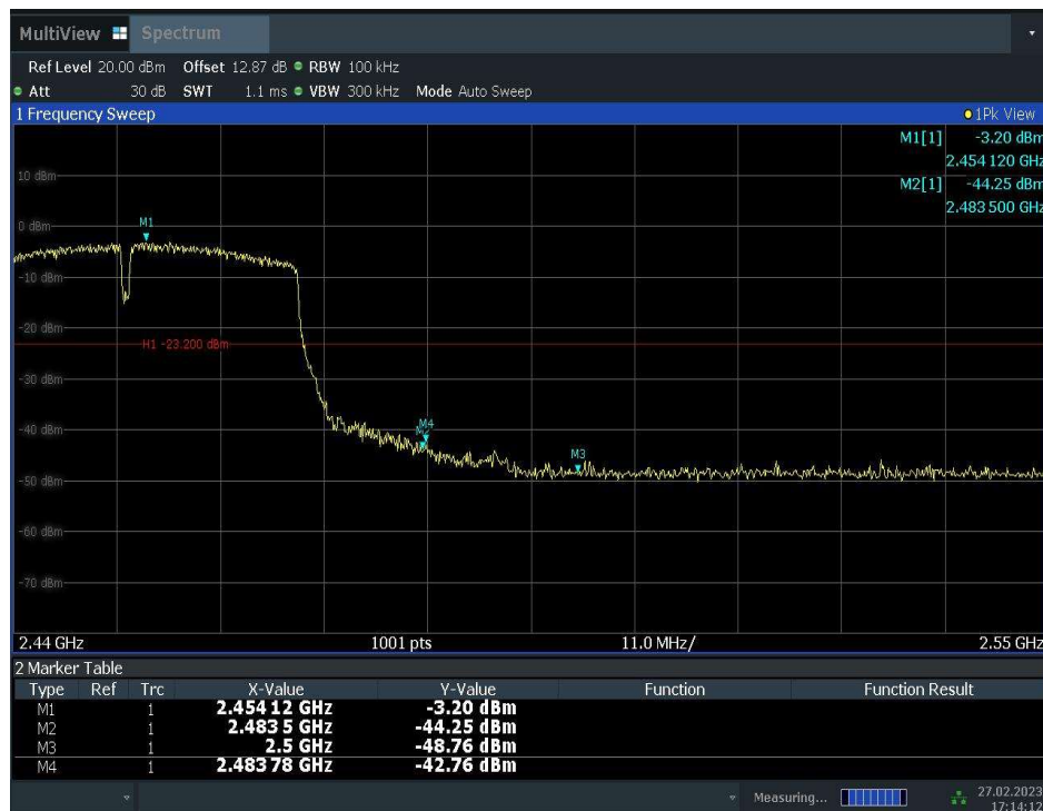
Fig.A.5.8 Band Edges (802.11n-HT40, Ch 9)
