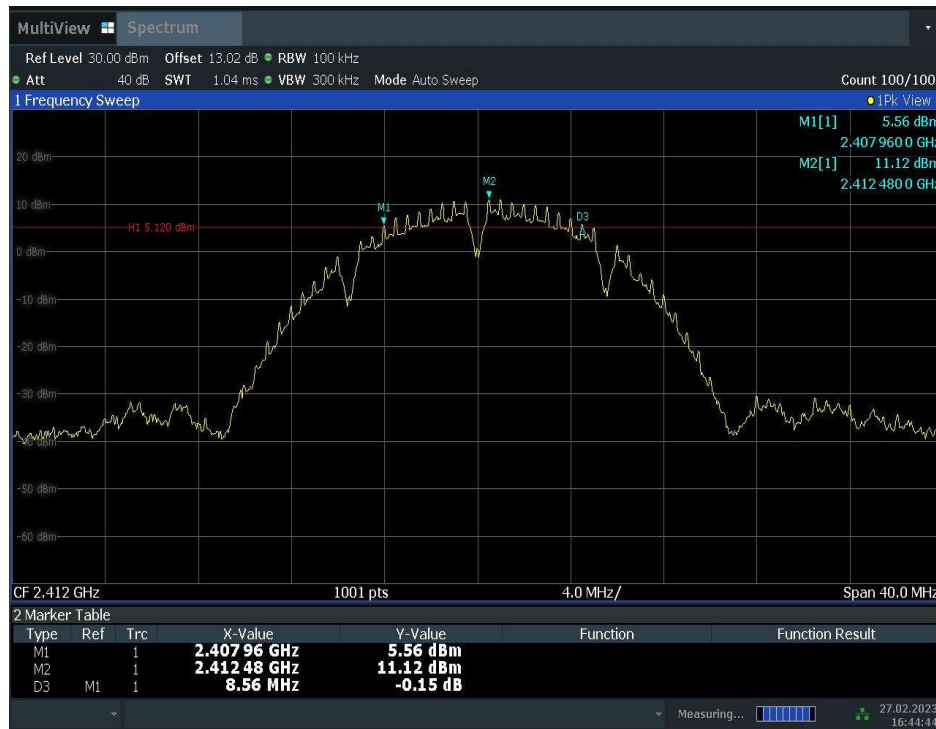
Fig.A.4.1 Occupied 6dB Bandwidth(802.11b,Ch 1)
