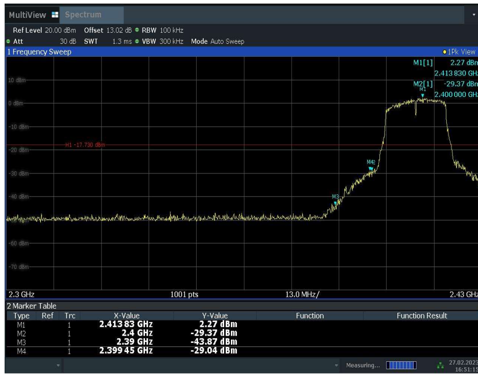
Fig.A.5.3 Band Edges (802.11g, Ch 1)
