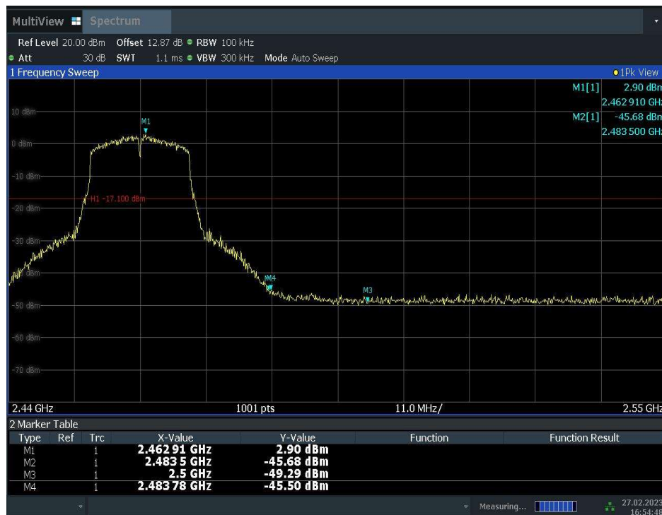
Fig.A.5.4 Band Edges (802.11g, Ch 11)
