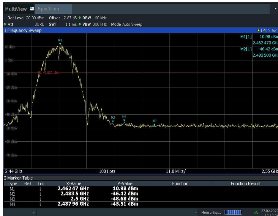
Fig.A.5.2 Band Edges (802.11b, Ch 11)
