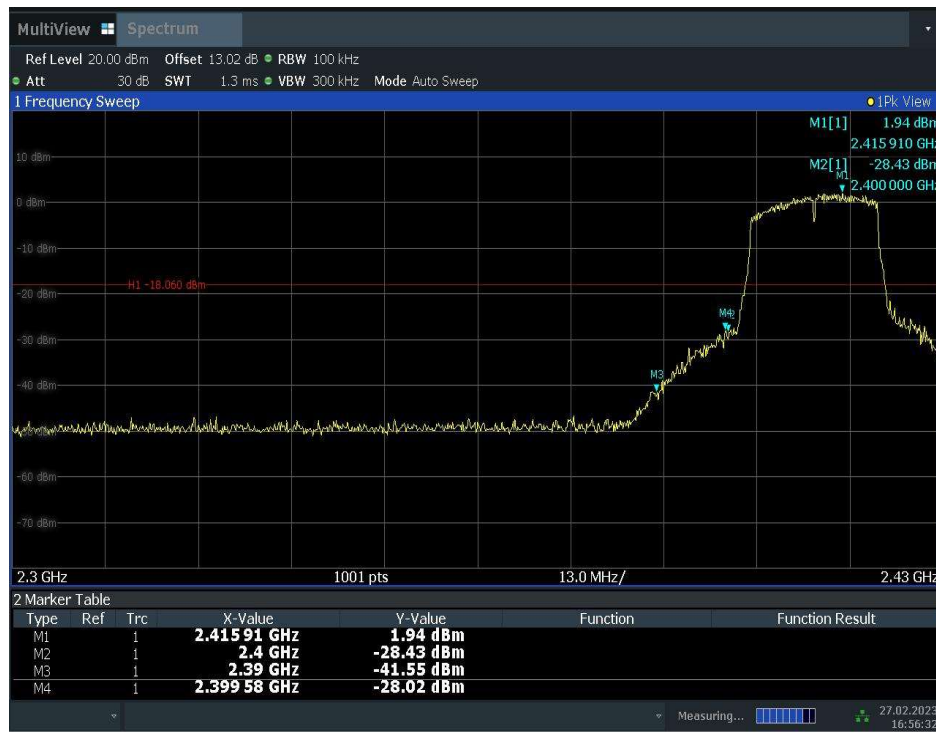
Fig.A.5.5 Band Edges (802.11n-HT20, Ch 1)
