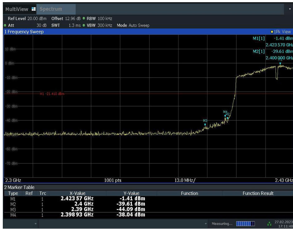
Fig.A.5.7 Band Edges (802.11n-HT40, Ch 3)
