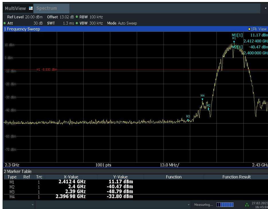
Fig.A.5.1 Band Edges (802.11b, Ch 1)
