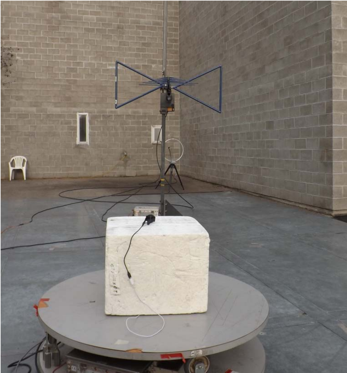
Figure E20.3 – Setup Photo – Radiated Measurements 30 – 1000MHz
