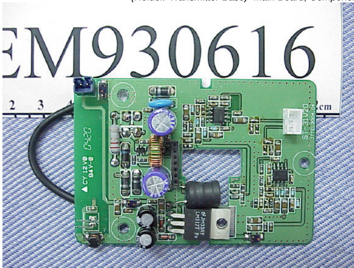
Photo 7 (Holder/ Transmitter Base) Main Board, Component Side
