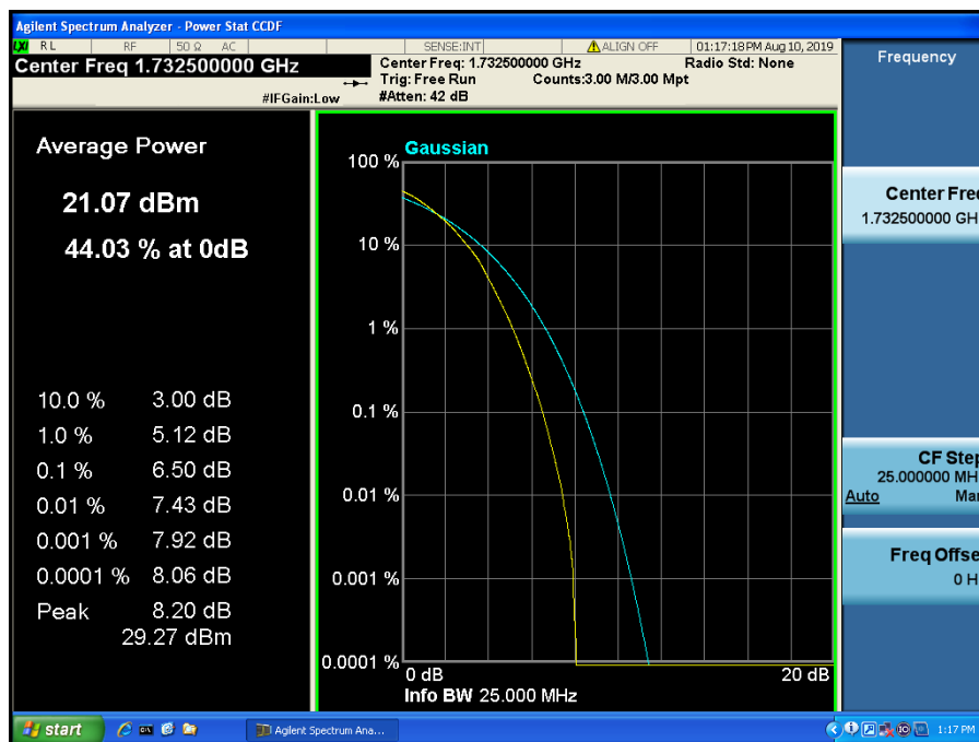
LTE Band 4 / 15 MHz / 64QAM - RB Size 75
