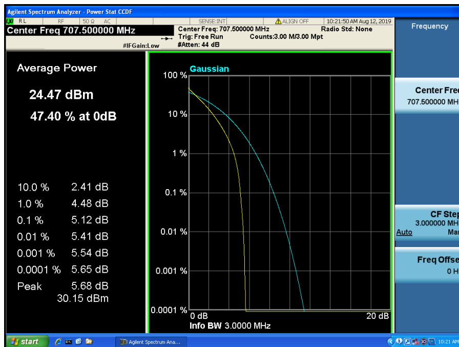
LTE Band 12 / 3 MHz / QPSK - RB Size 15
