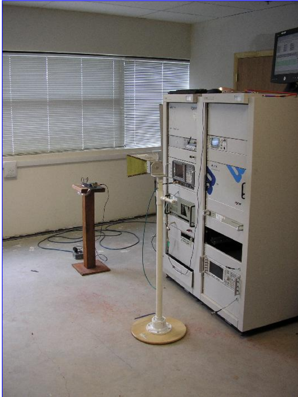
Photograph 1. Radiated Spurious Emissions Test Set Up
