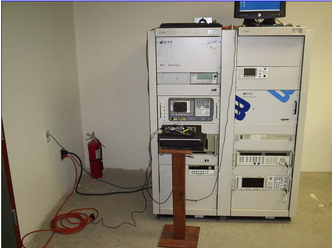
Photograph 2. Output Power; Test Setup
