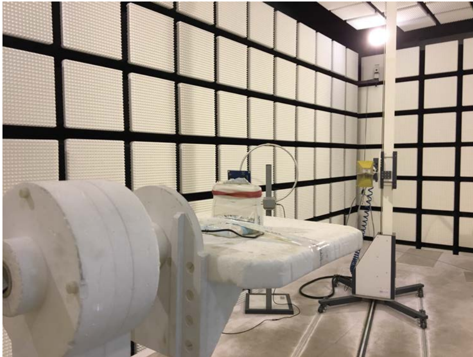
Photo 5: radiated emission above 1GHz
