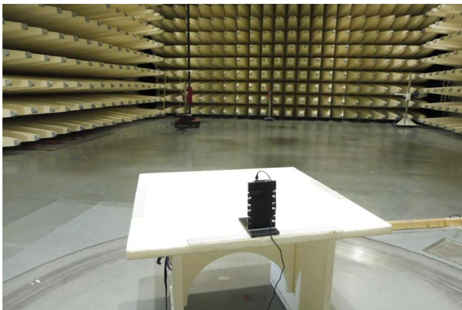
Photo 2: radiated emission 30MHz - 1GHz
