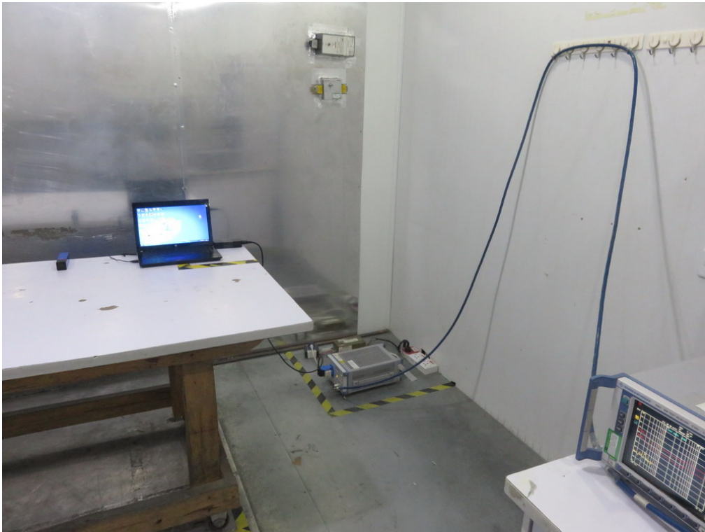
FCC RADIATED EMISSION TEST SETUP
