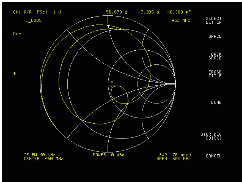
**450 MHz Body Liquid Validation, Ambient Temp=23 Deg C , Liquid Temp=22 Deg C , 9/27/2004**
