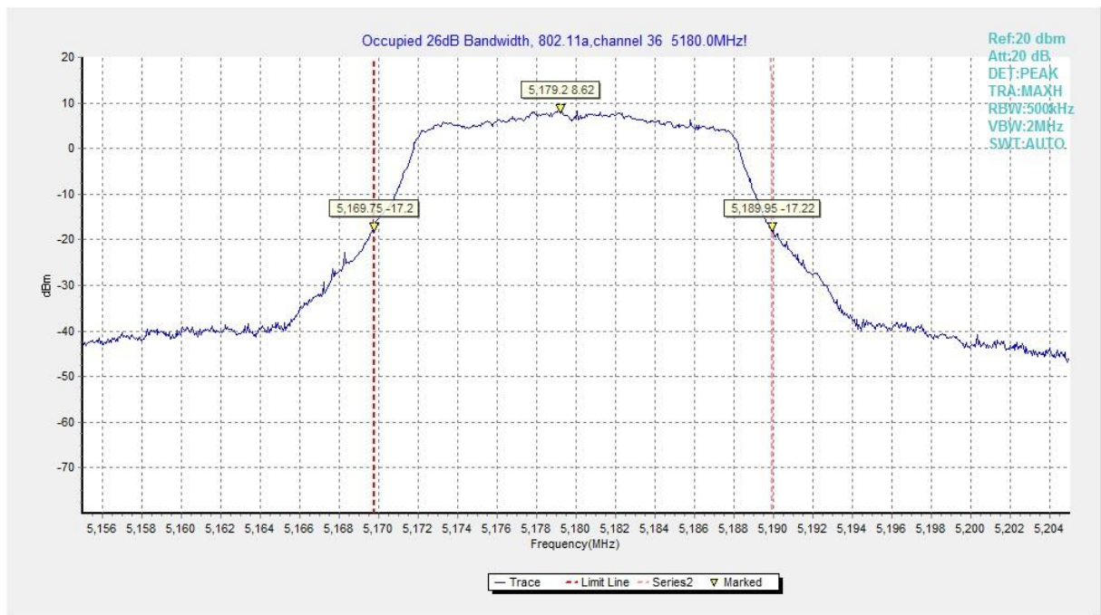
Fig. 1 Occupied 26dB Bandwidth (802.11a, 5180MHz)
