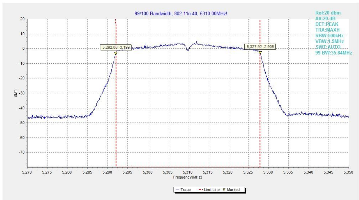
Fig. 42 99% Occupied Bandwidth (802.11n-HT40, 5310MHz)
