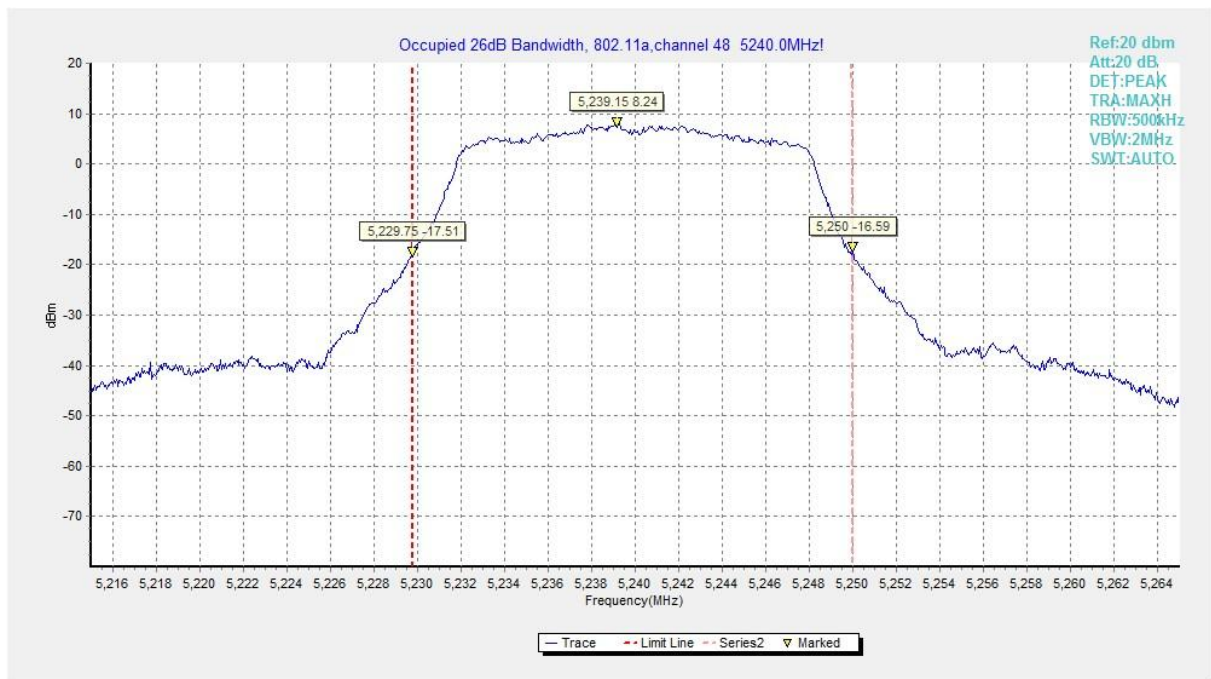
Fig. 3 Occupied 26dB Bandwidth (802.11a, 5240MHz)
