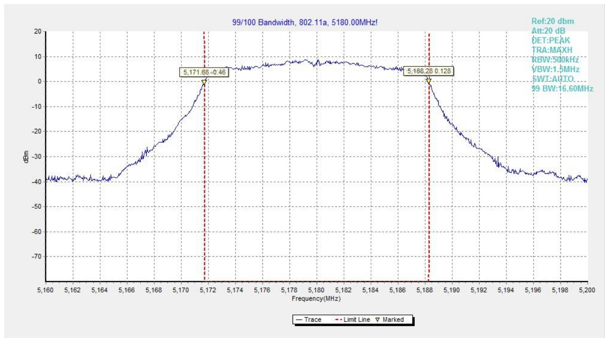
Fig. 27 99% Occupied Bandwidth (802.11a, 5180MHz)
