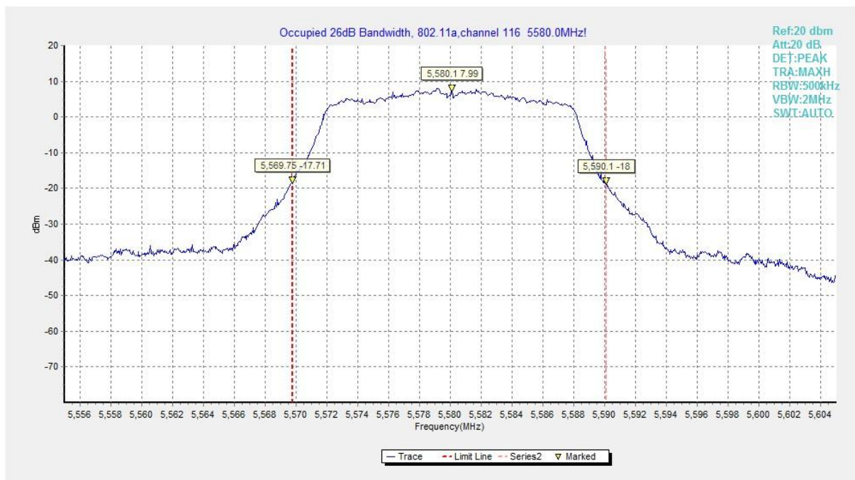
Fig. 8 Occupied 26dB Bandwidth (802.11a, 5580MHz)
