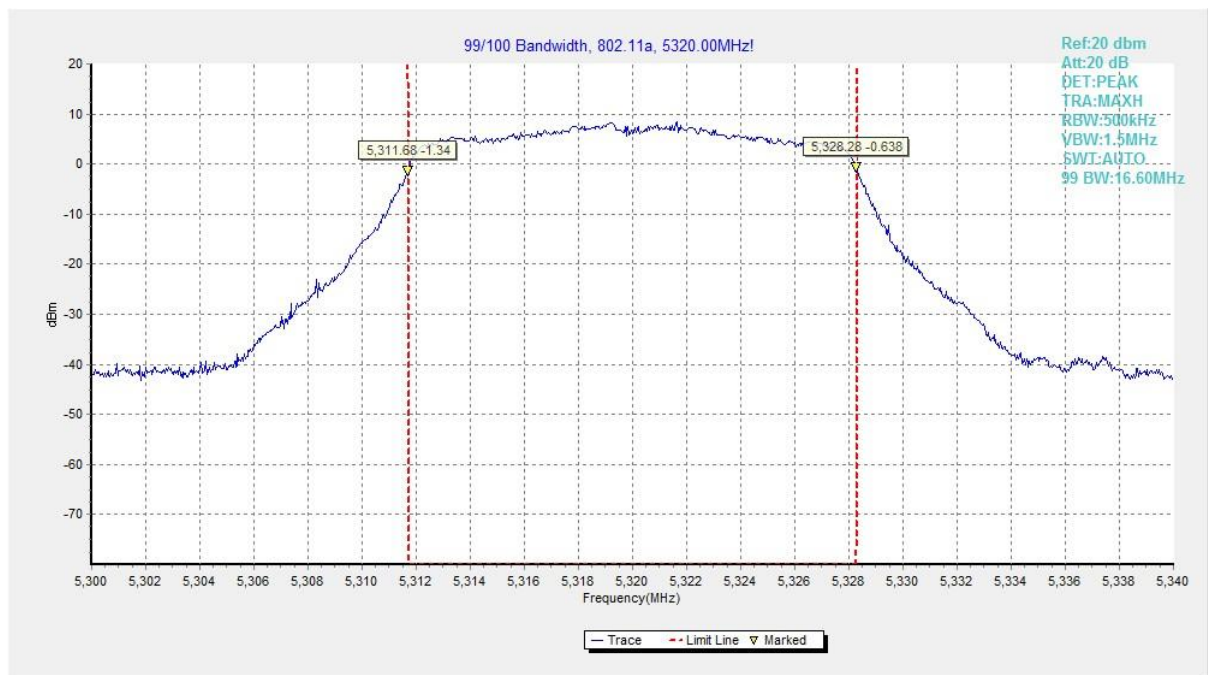
Fig. 32 99% Occupied Bandwidth (802.11a, 5320MHz)
