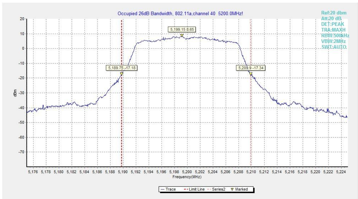
Fig. 2 Occupied 26dB Bandwidth (802.11a, 5200MHz)
