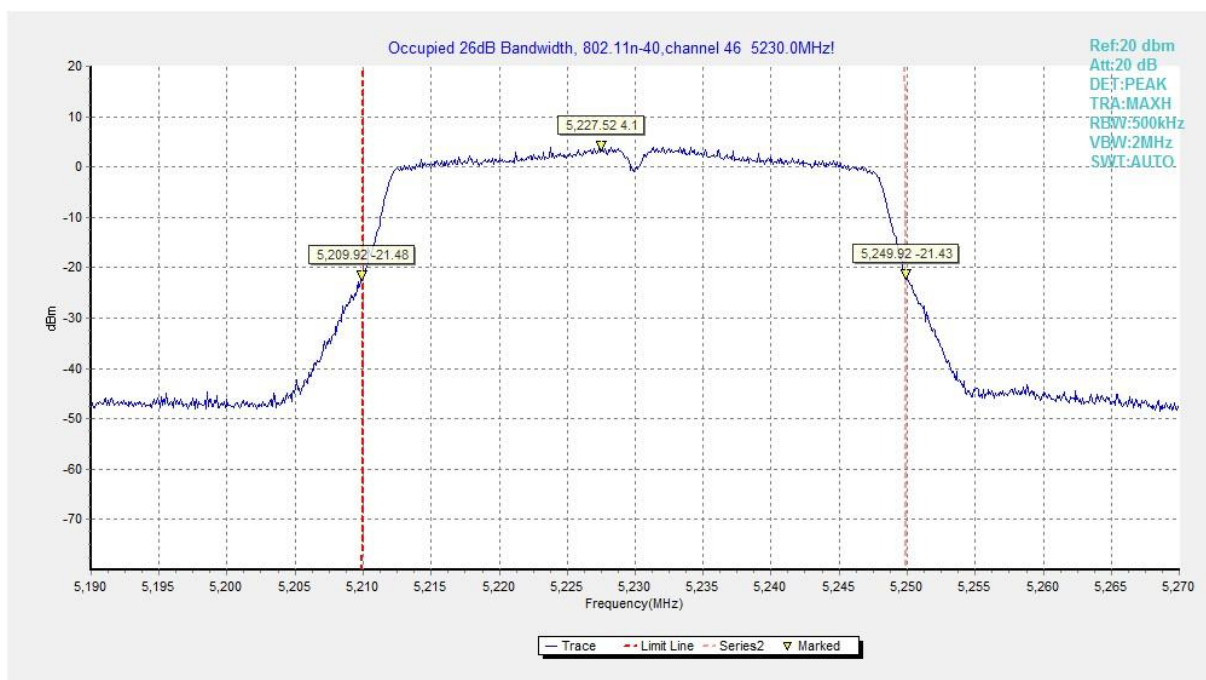
Fig. 11 Occupied 26dB Bandwidth (802.11n-HT40, 5230MHz)
