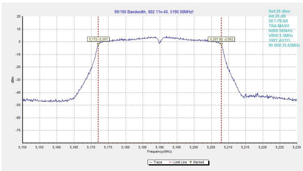
Fig. 39 99% Occupied Bandwidth (802.11n-HT40, 5190MHz)
