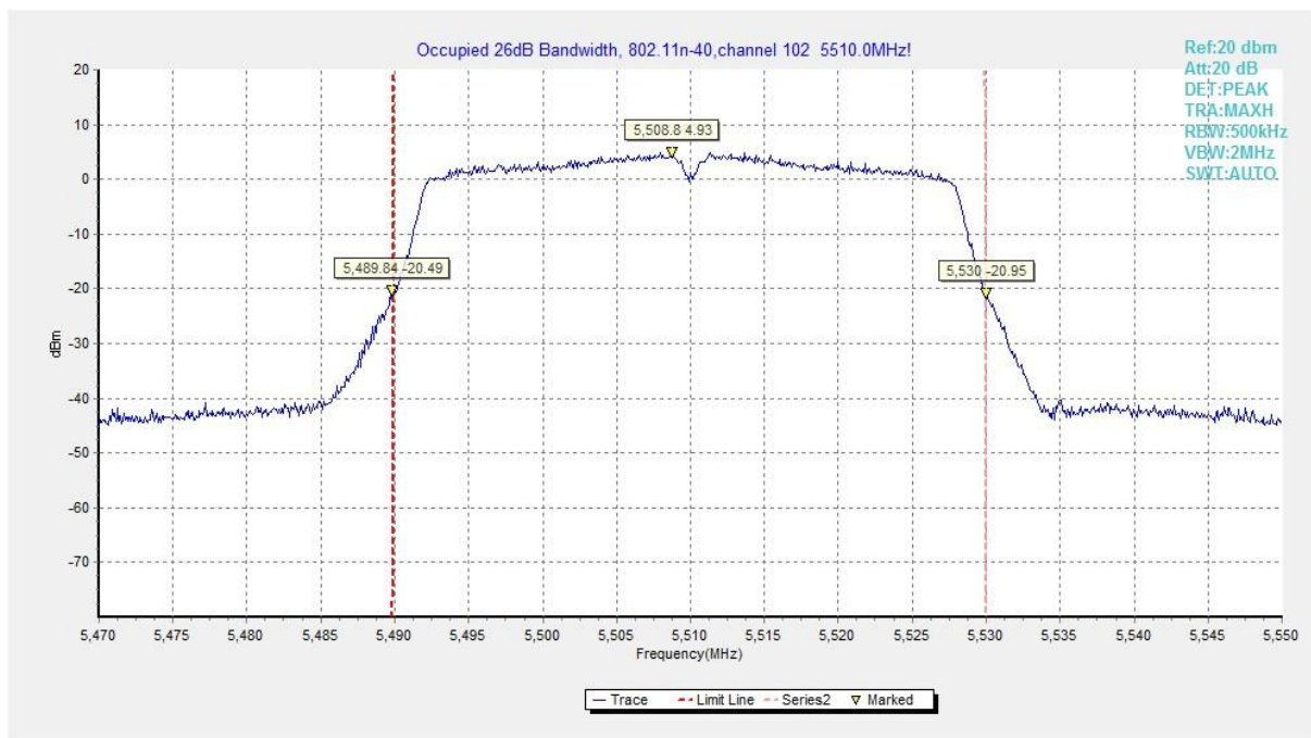
Fig. 14 Occupied 26dB Bandwidth (802.11n-HT40, 5510MHz)
