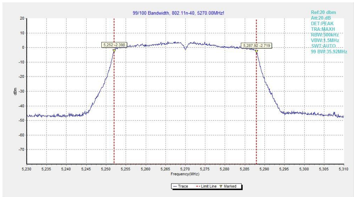
Fig. 41 99% Occupied Bandwidth (802.11n-HT40, 5270MHz)
