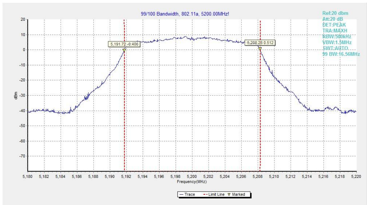
Fig. 28 99% Occupied Bandwidth (802.11a, 5200MHz)
