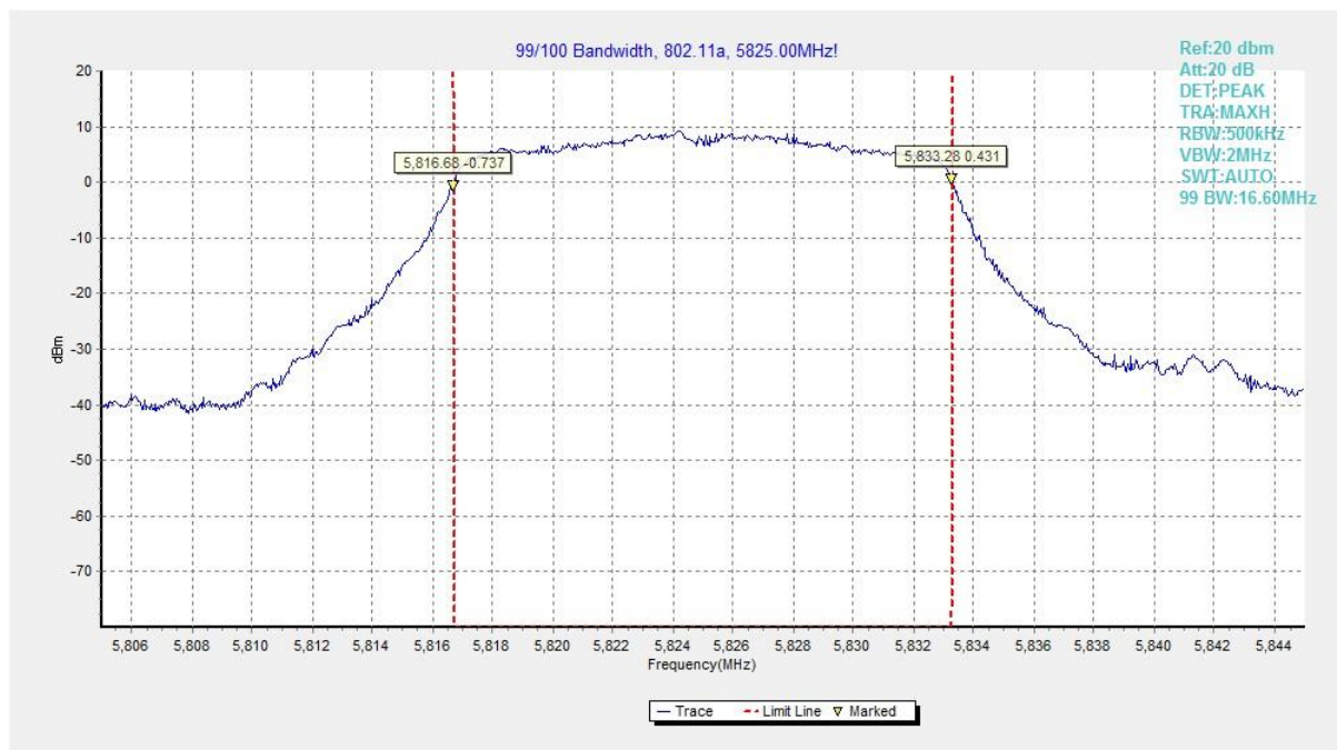
Fig. 38 99% Occupied Bandwidth (802.11a, 5825MHz)
