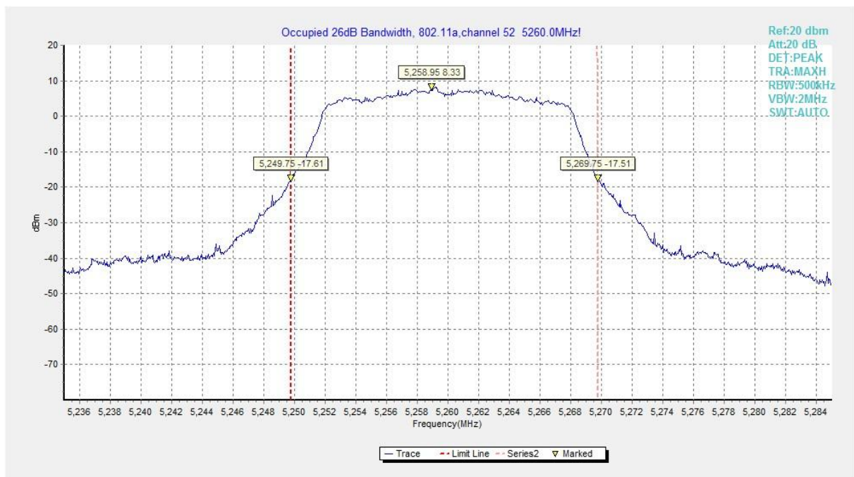
Fig. 4 Occupied 26dB Bandwidth (802.11a, 5260MHz)
