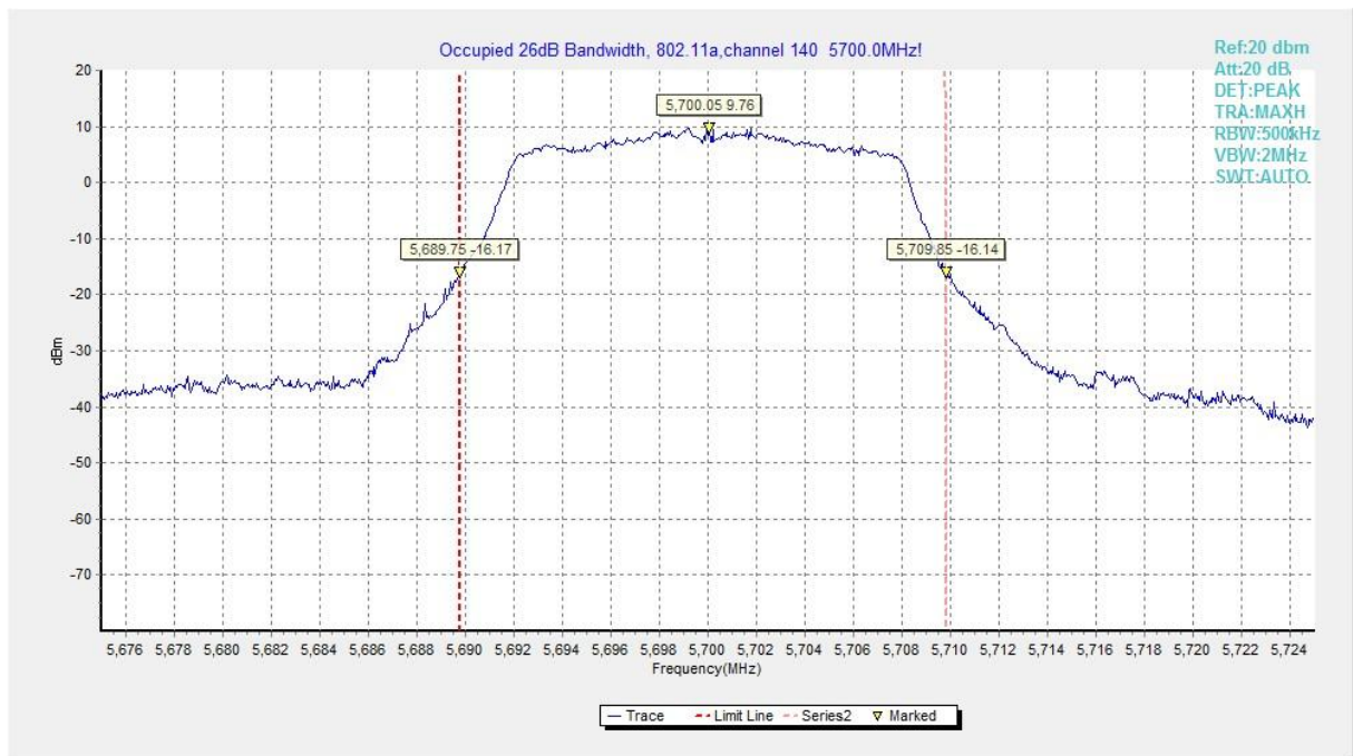
Fig. 9 Occupied 26dB Bandwidth (802.11a, 5700MHz)
