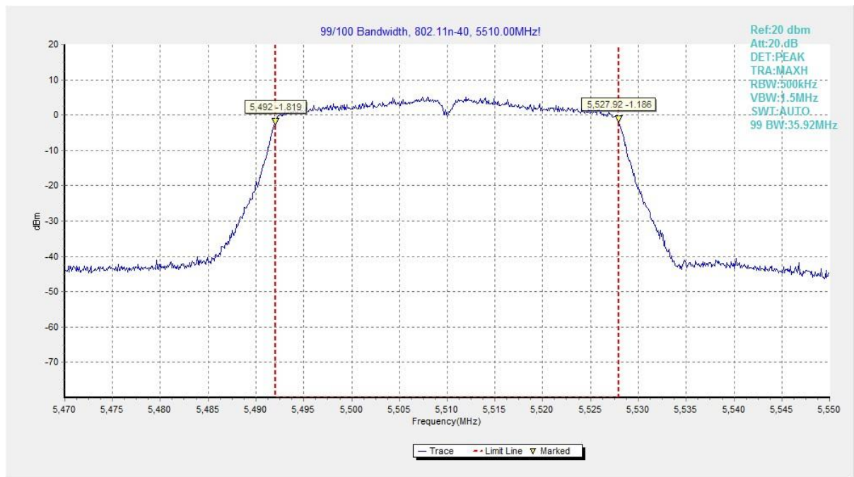
Fig. 43 99% Occupied Bandwidth (802.11n-HT40, 5510MHz)
