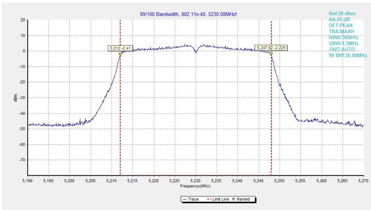
Fig. 40 99% Occupied Bandwidth (802.11n-HT40, 5230MHz)
