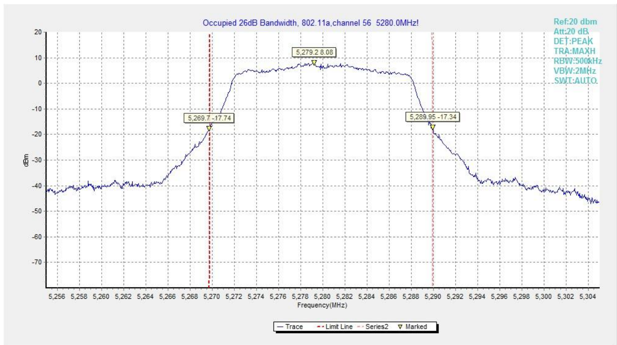
Fig. 5 Occupied 26dB Bandwidth (802.11a, 5280MHz)
