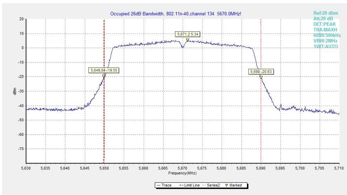
Fig. 15 Occupied 26dB Bandwidth (802.11n-HT40, 5670MHz)
