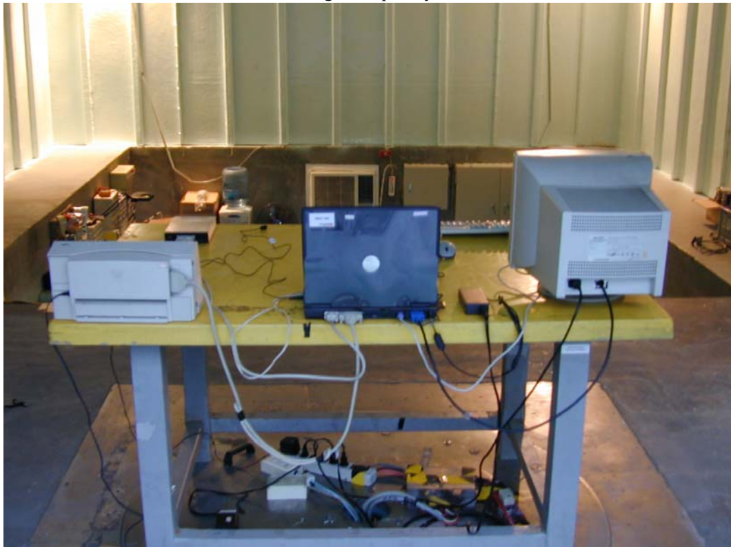
Back View of High Frequency Radiated Test
