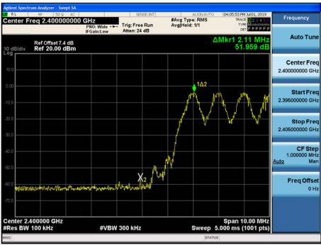
Test Plots with hopping (GFSK)
