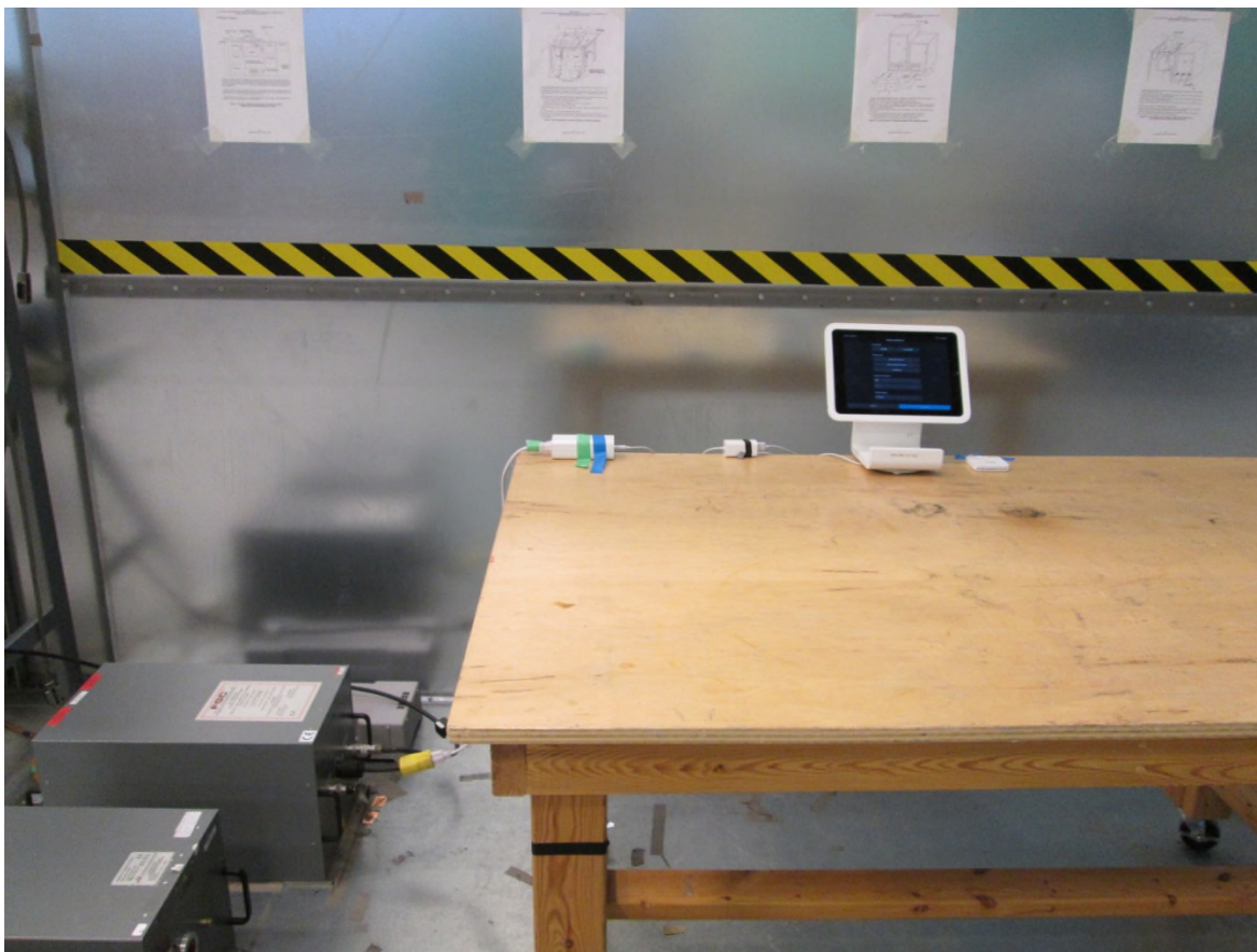
Test setup photo 8 Power line conducted emissions measurements
