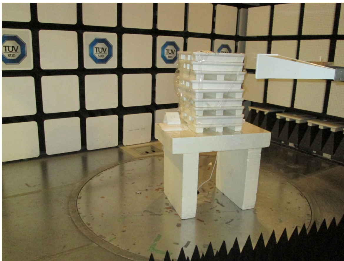
Test setup photo 5 Radiated measurements, 10 GHz – 18 GHz
