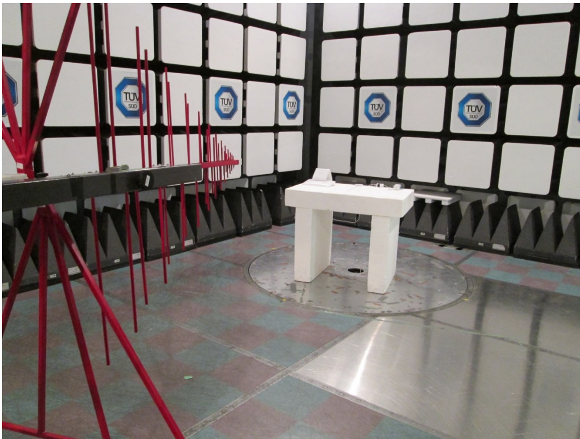
Test setup photo 2 Radiated measurements, 30 MHz – 1 GHz
