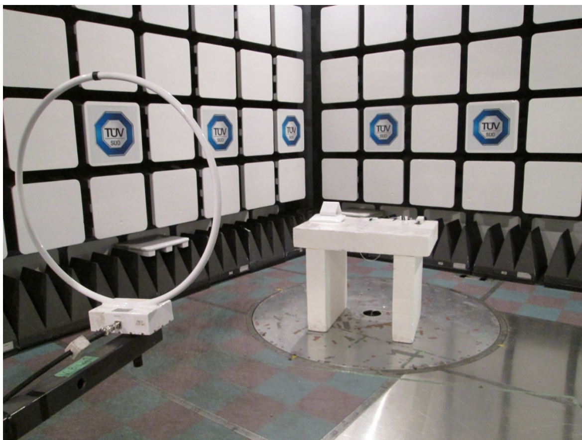
Test setup photo 1 Radiated measurements, 9 kHz – 30 MHz
