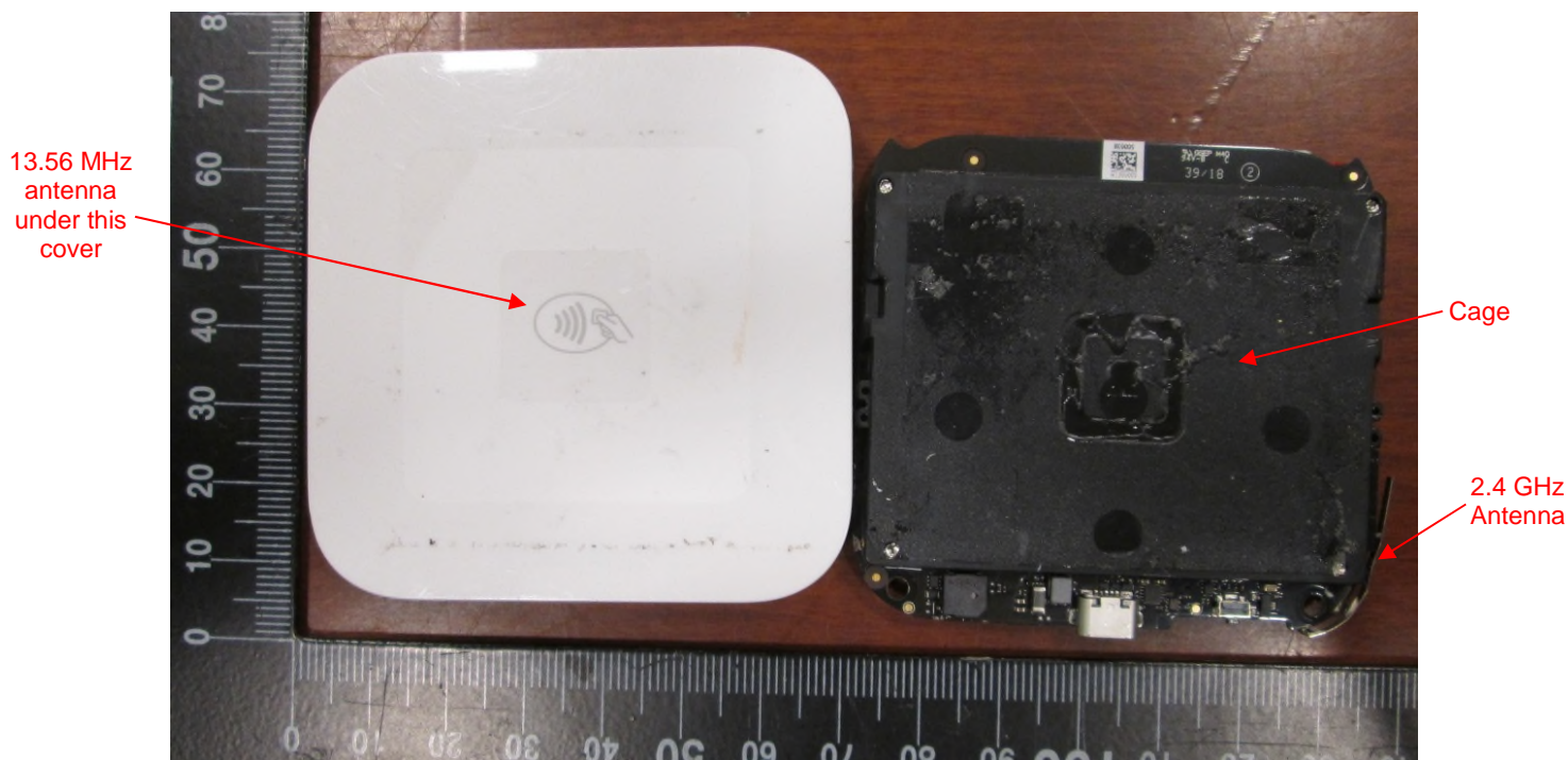
EUT – Internal view 2 PCB removed from enclosure
