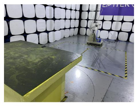
Spurious Emission Test Setup (Above 1GHz)
