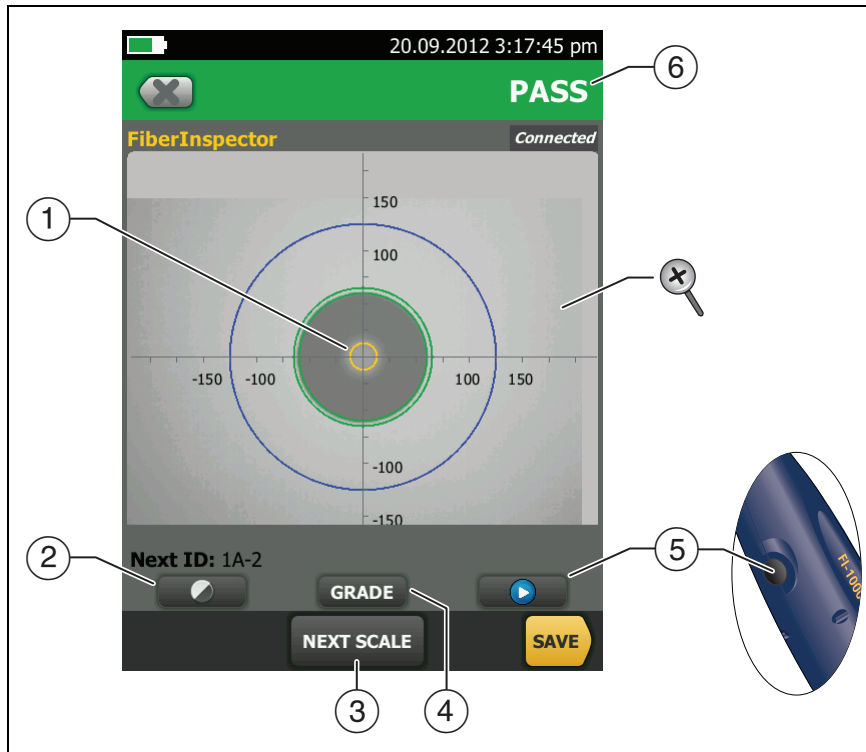
Figure 38. FiberInspector Image with Manual Grading Selected
