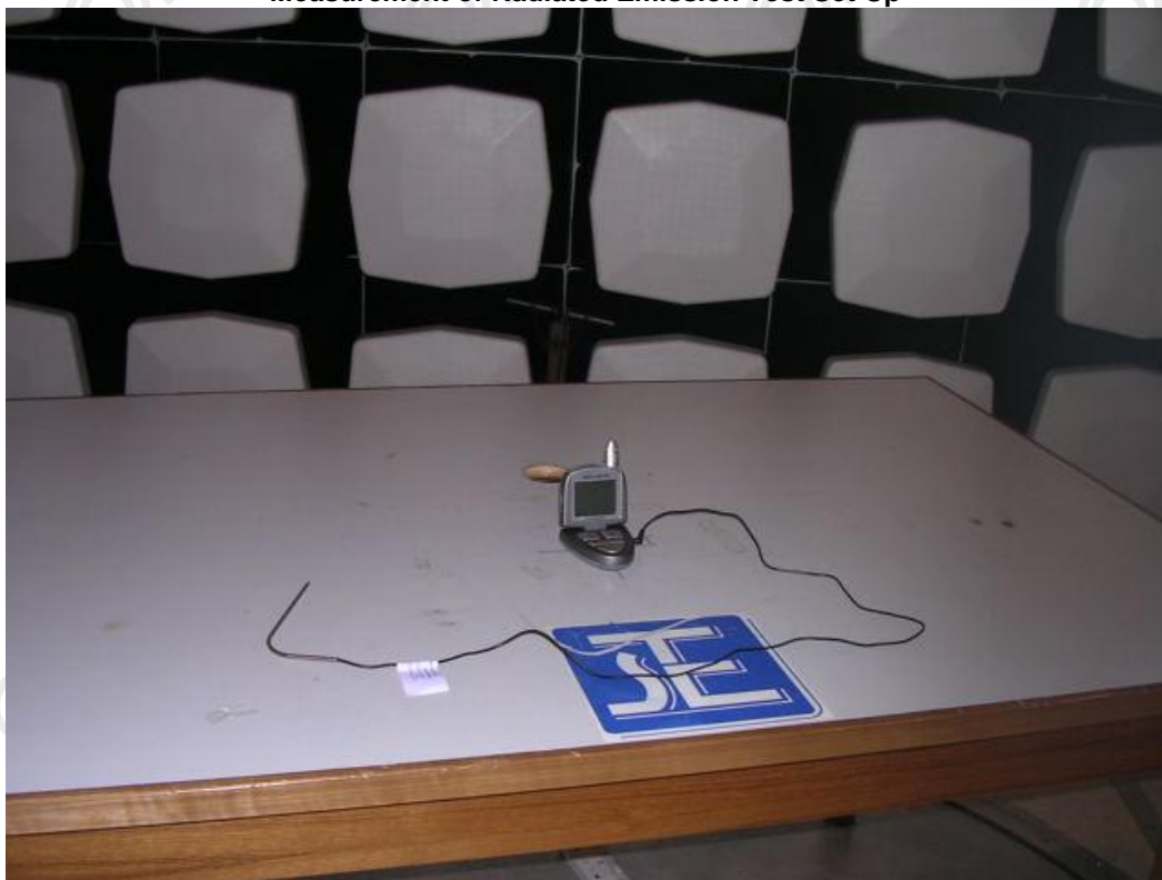
Measurement of Radiated Emission Test Set Up
