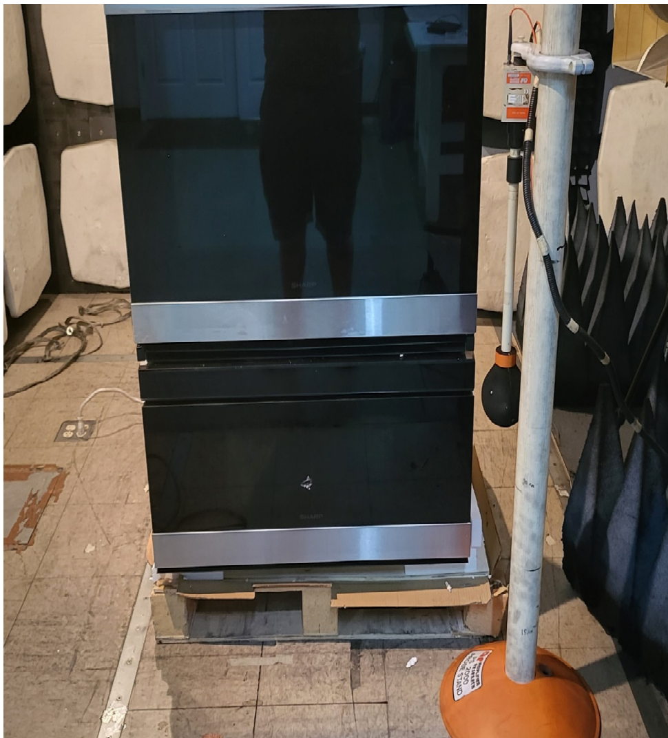
Figure 6. Radiation Leakage w/ RF Probe
