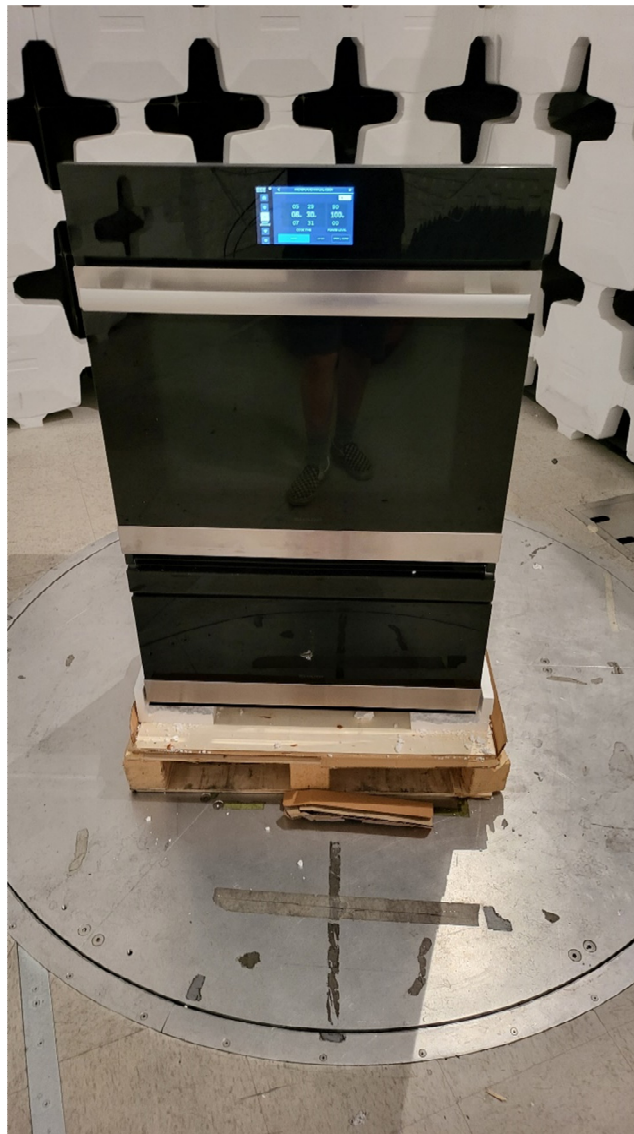
Figure 1. Radiated Emissions Measurement Photo (Front View)
