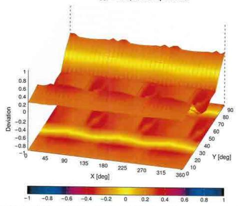
Probe isotropy for  $E_{tot}$ : probe rotated  $\phi=0^\circ$  to 360°, tilted from field propagation direction  $\vec{k}$  Parallel to the field propagation ( $\psi=0^\circ-90^\circ$ ) at 30 GHz: deviation within  $\pm 0.40$  dB Parallel to the field propagation ( $\psi=0^\circ-90^\circ$ ) at 60 GHz: deviation within  $\pm 0.39$  dB
