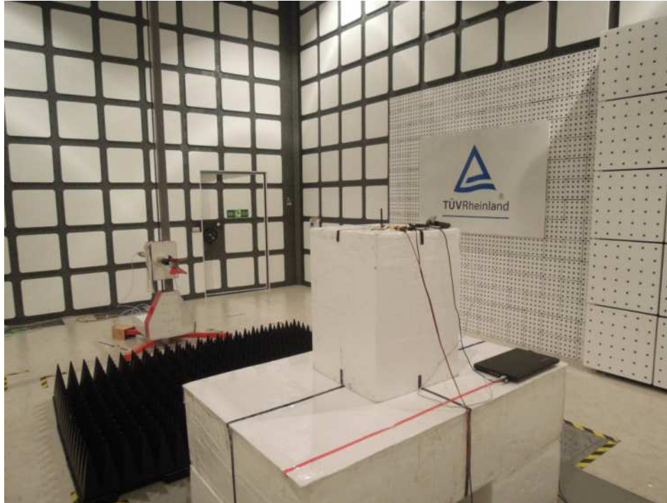
Photograph 23: Set-up for Spurious Emissions (Front View)- RFDPA870920IMLB301 - ANT
