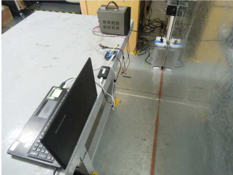
Photograph 36: Set-up for Mains Conducted testing (Back View)
