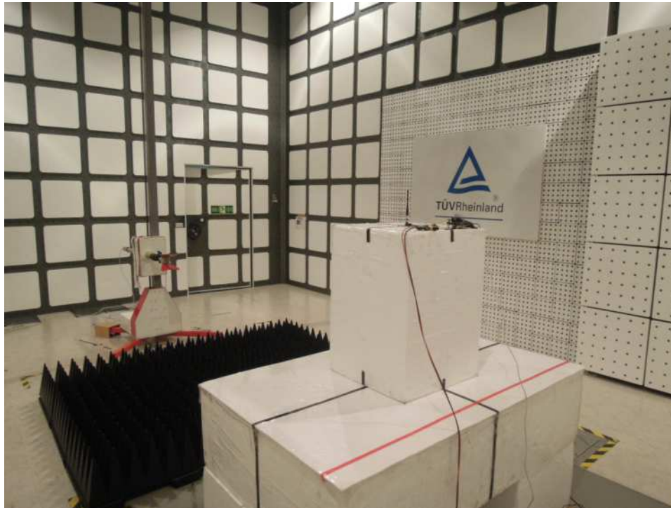
Photograph 5: Set-up for Spurious Emissions (Back View 3)- RFA-02-5-C7H1-ANT
