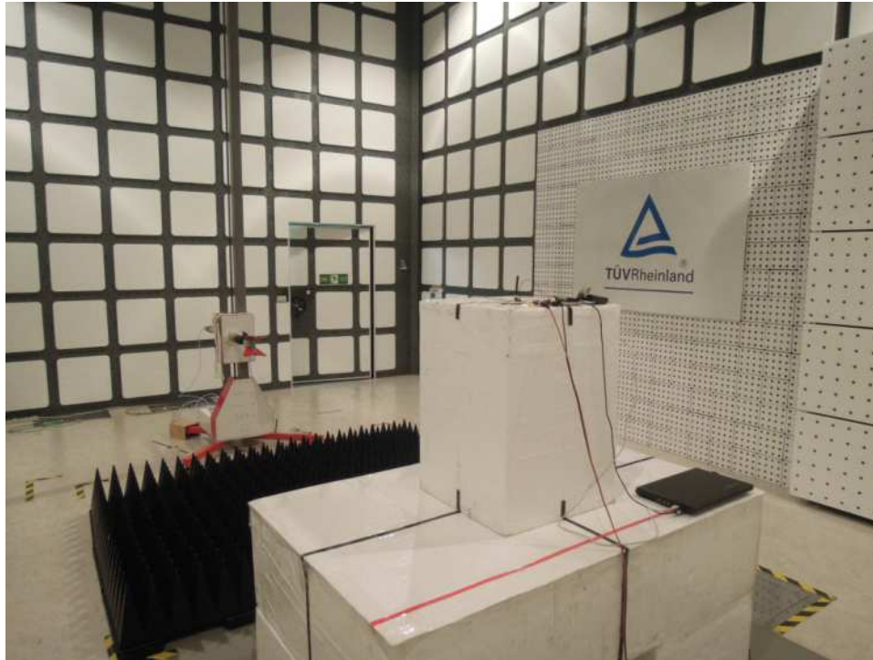
Photograph 25: Set-up for Spurious Emissions (Front View)- RFA-02-3-C5H1 -ANT
