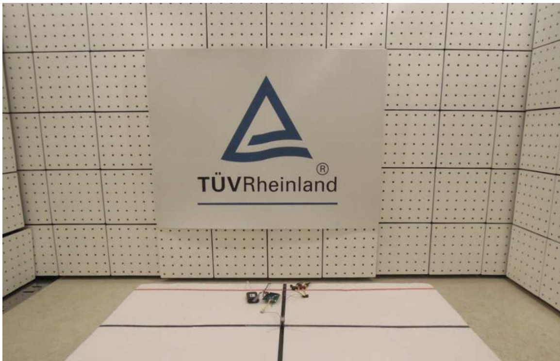
Photograph 1: Set-up for Spurious Emissions (Front View 1)- RFA-02-5-C7H1-ANT
