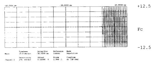
Trigger mode : Edge On Positive Edge Of Chan2 Trigger Level Chan2 - 412.500 mV (noise reject ON) Holdoff = 40.000 ns
