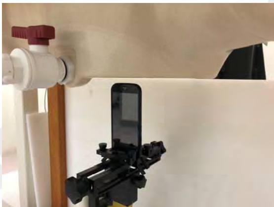
Fig.11 EUT Bottom side to flat phantom
