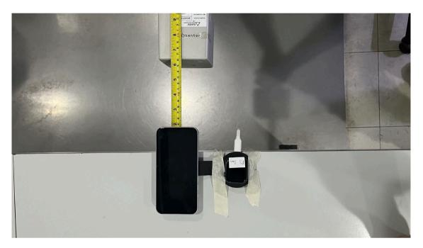
The definition of location for RF exposure test
