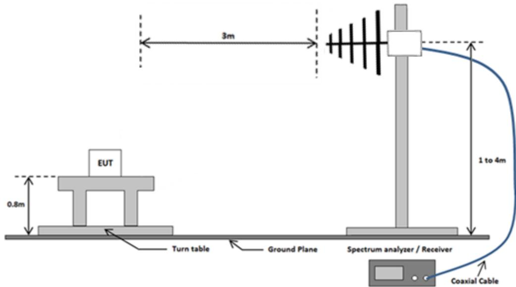
**Radiated emissions test setup above 1 GHz**
