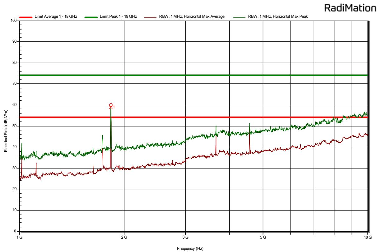
**Note:** The harmonics seen in the plots above are falls inside of restricted bands of operation defined in Part 15.205 of the FCC regulation. Thus as described in FCC Part 15.247 sub-section (d) the actual applicable limit shall be 20 dB lower of the actual transmitter peak value which is 94.39 dB $\mu$ V/m for this case.
