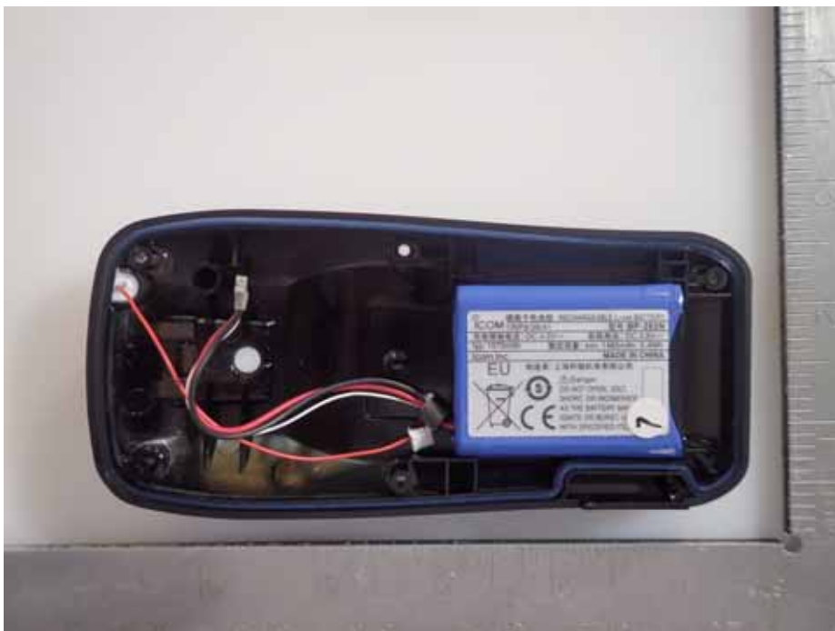
Li-ion Chargeable Battery (M/N: BP-282N, 4.2V, 1570mAh)
