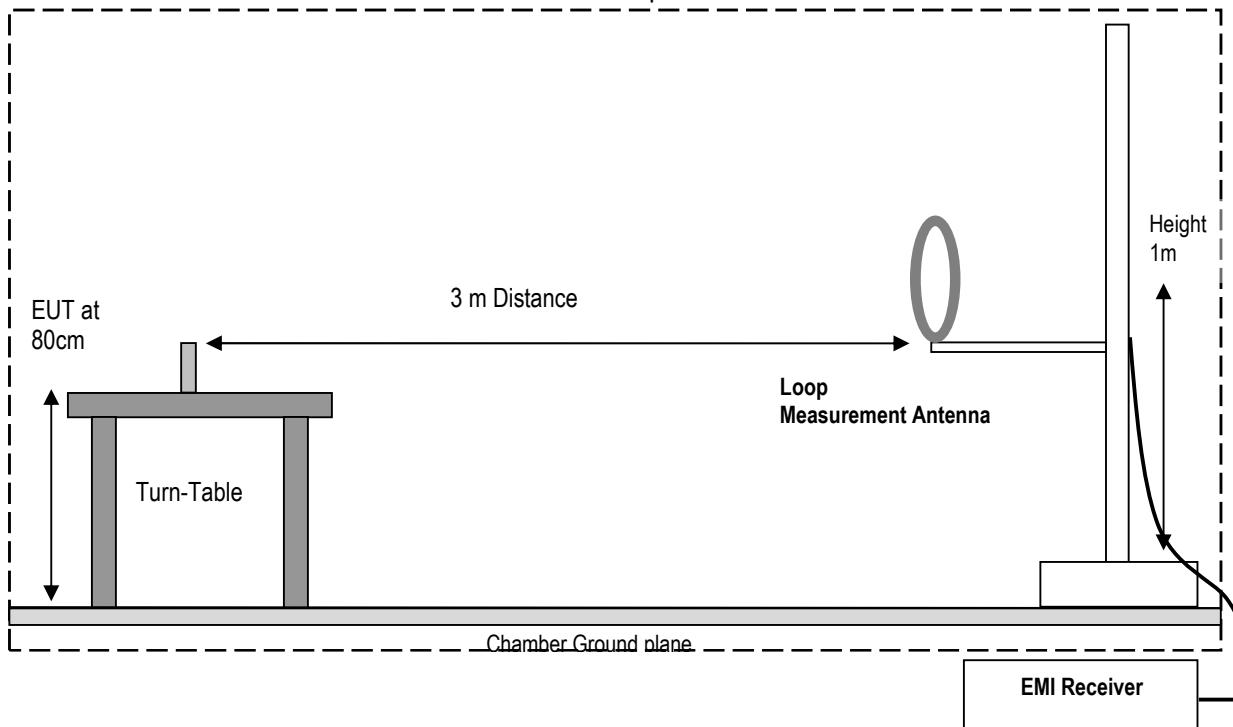
Radiated Emissions Test Setup 30MHz-1GHz Measurements
