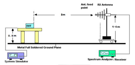
For radiated test from above 1GHz
