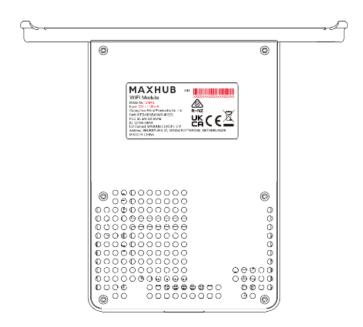
The label is attached to the back of the device with a permanent adhesive.
